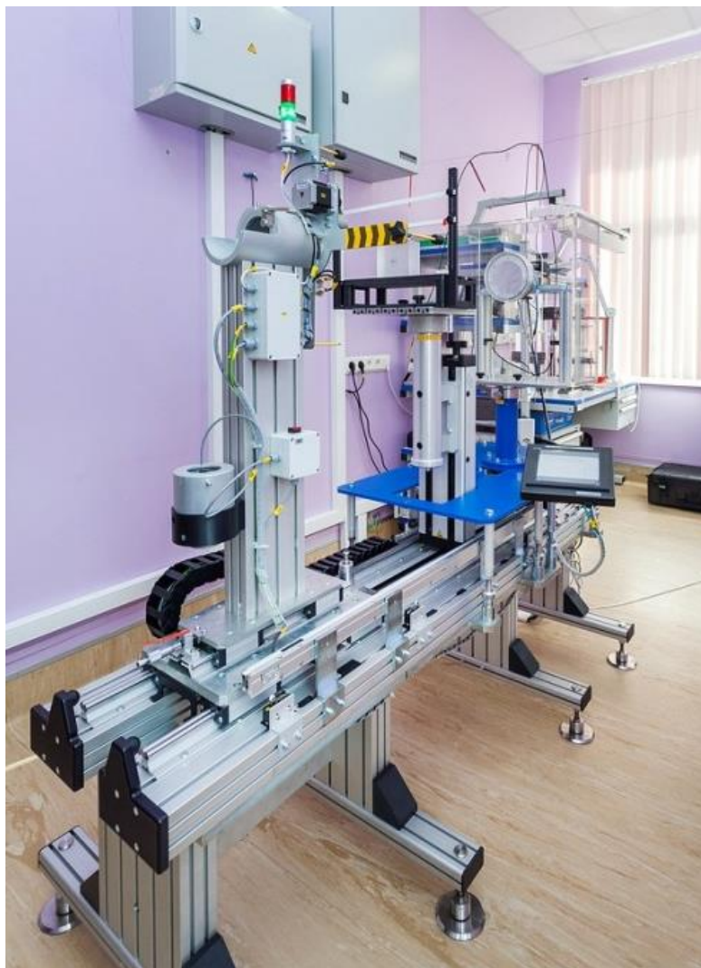
Fig. 2. UEDAB-1 facility for beta radiation absorbed dose to tissue measurements
