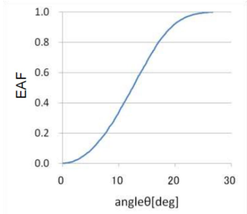
$$EAF(\theta') = \frac{\int_0^{2\pi} \int_0^{\theta'} I(\theta, \varphi) \cdot \frac{\sin(\theta)}{\cos^3(\theta)} \cdot d\theta \cdot d\varphi}{\int_0^{2\pi} \int_0^{\theta_{\max}} I(\theta, \varphi) \cdot \frac{\sin(\theta)}{\cos^3(\theta)} \cdot d\theta \cdot d\varphi}$$
