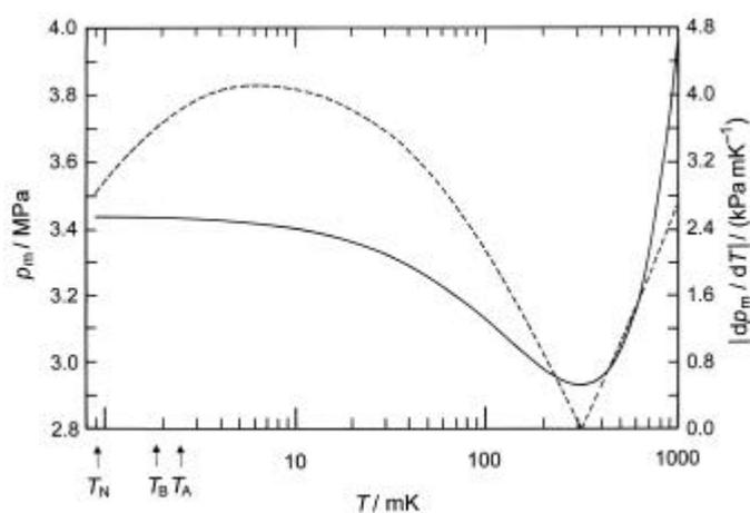
Figure : The  $^3\text{He}$  melting pressure  $p$  (full line) and the absolute value of the derivative  $dp/dT$  (dashed line) vs. temperature.  $T_N$ ,  $T_B$  and  $T_A$  indicate the temperatures of three phase transitions in solid or liquid  $^3\text{He}$ .
