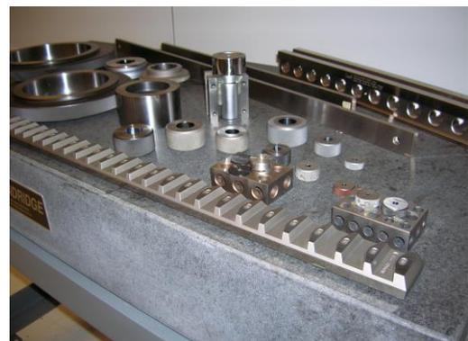
**Figure 4.** Step gages, ring gages, plugs, and long end standards being measured on a CMM. The flexibility of a CMM might eventually enable a shift away from some of the traditional artefact standards and the key comparison portfolio will evolve accordingly.
