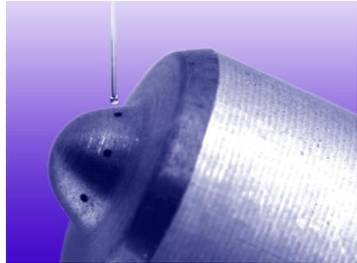
**Figure 6.** Micro-probe measures 130  $\mu\text{m}$  diameter holes in an advanced fuel injector.
