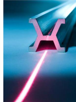
**Figure 1.** The metre, originally defined by a length marked on a bar such as shown in the background, is currently defined via the speed of light and realized via the wavelength and frequency of lasers, as illustrated by the laser beam in the foreground.
