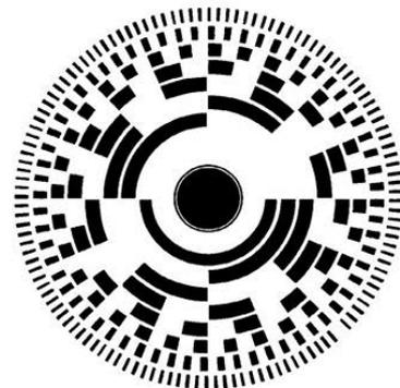
**Figure 5.** Angle encoders are playing an increasing role in angle metrology.
