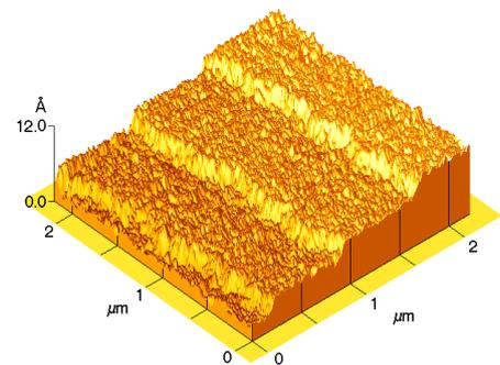
**Figure 3.** Single-atom steps on a silicon (111) lattice.
