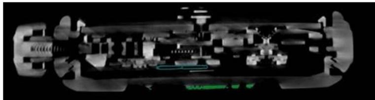
**Figure 7.** X-ray CT allows measurements of hidden features with high data density, as in this cross-sectional image of a watch.
