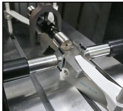
I studied and performed this calibration with ULM and CMM. The method used in this calibration is the two ball method and three wire method. During the training, I studied the theoretical aspects of threaded gauge calibrations, calibration procedures, work instructions, document standards, best practices and factors that contribute to uncertainties of measurement. I also learned about pitch diameter calculations and produced uncertainty calculations for this calibration.
