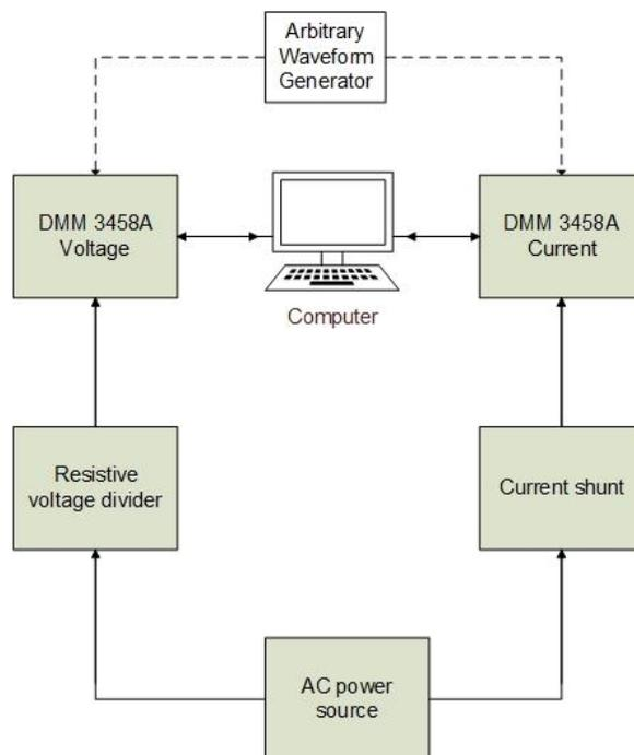
Figure 2. Block diagram of DSWM
