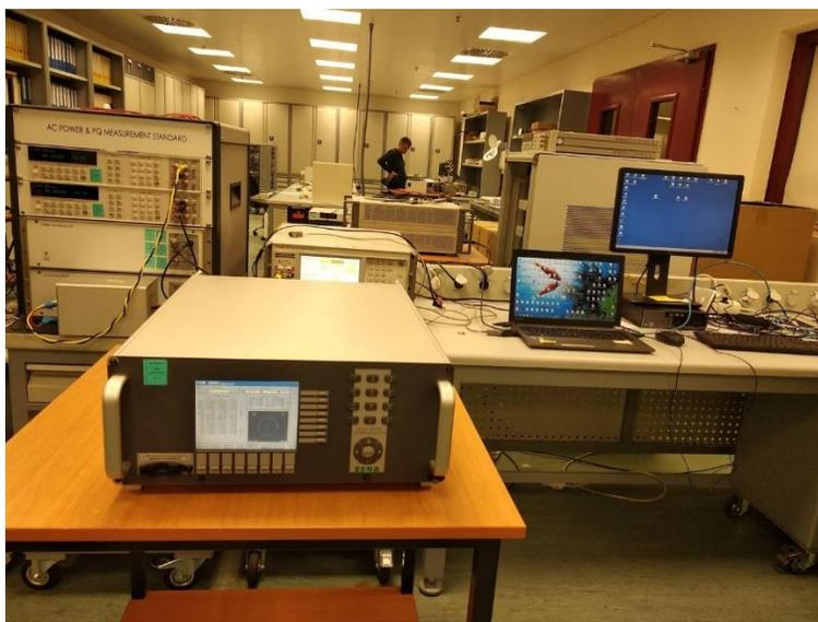
Figure 1. Calibration of ZERA COM3003 using DSWM
