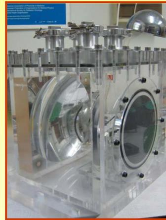
The calorimeter in its vacuum chamber.
