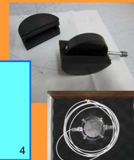
Ionization chamber in graphite jacket ...and water phantom.
