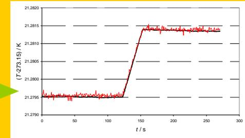
Temperatures measured before, during and after irradiation of the calorimeter in a 6 MV accelerator beam, demonstrating quasi-adiabatic behaviour. The black curve represents the temperature of the calorimeter core using two thermistors in opposite arms of a d.c. Wheatstone bridge, while the red curve shows the temperature of the jacket. The jacket is measured using a single thermistor and an ohm-meter and the signal is therefore noisier than that of the core.
