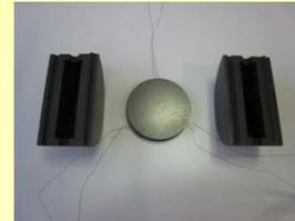
The calorimeter was designed to minimize the temperature difference between the core and jacket, and to reduce as far as possible heat exchange, notably radiative heat transfer, between the jacket and its surroundings. Non-graphite materials were kept to a minimum to reduce their effect on the temperature rise.
