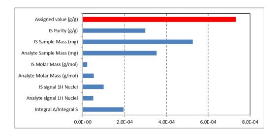
Figure 4 - Relative uncertainty components (in blue) for the uncertainty in the assigned purity value (in red) for DMSO<sub>2</sub> using MA as ISRM in D<sub>2</sub>O.
