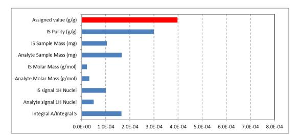
Figure 6 - Relative uncertainty components (in blue) for the uncertainty in the assigned purity value (in red) for DMTP when using MA as ISRM in DMSO- $d_6$ .
