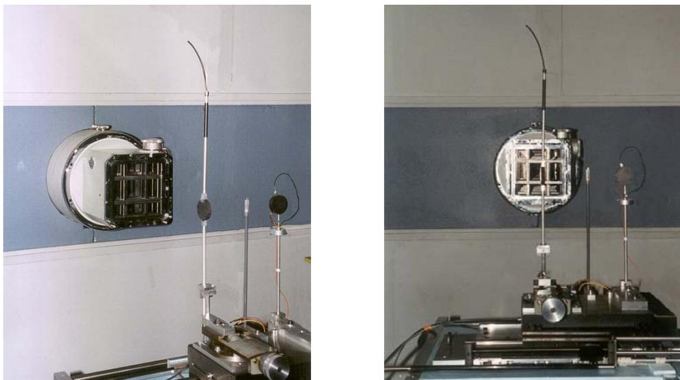
The stability of the PTB standards was confirmed by measurements made at the PTB after their return. Agreement for each standard was within  $3 \times 10^{-4}$  of its previous value.
