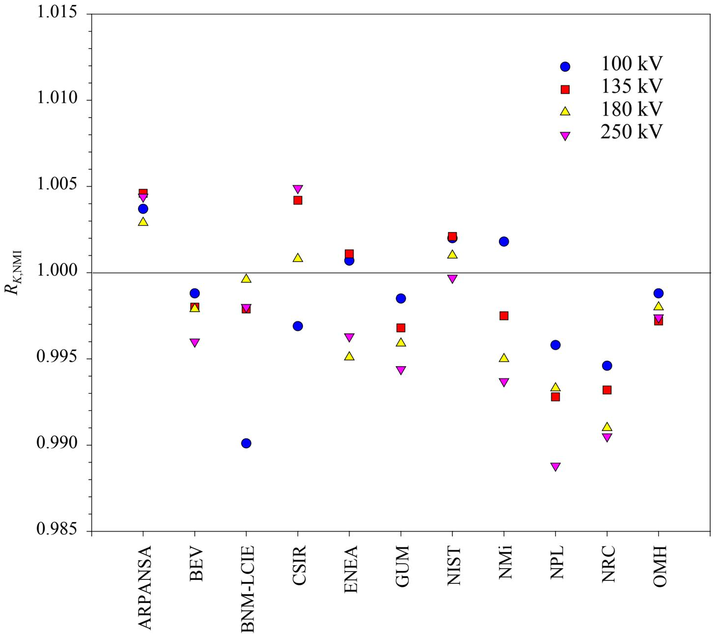
Figure 1. Results of BIPM medium-energy x-ray comparisons, expressed as the ratio  $R_{K,NMI}$  of the air-kerma rate determined by the standard of the national metrology institute (NMI) to that determined by the BIPM standard. For NMIs that have compared more than once with the BIPM, only the results of the most recent comparison are included.
