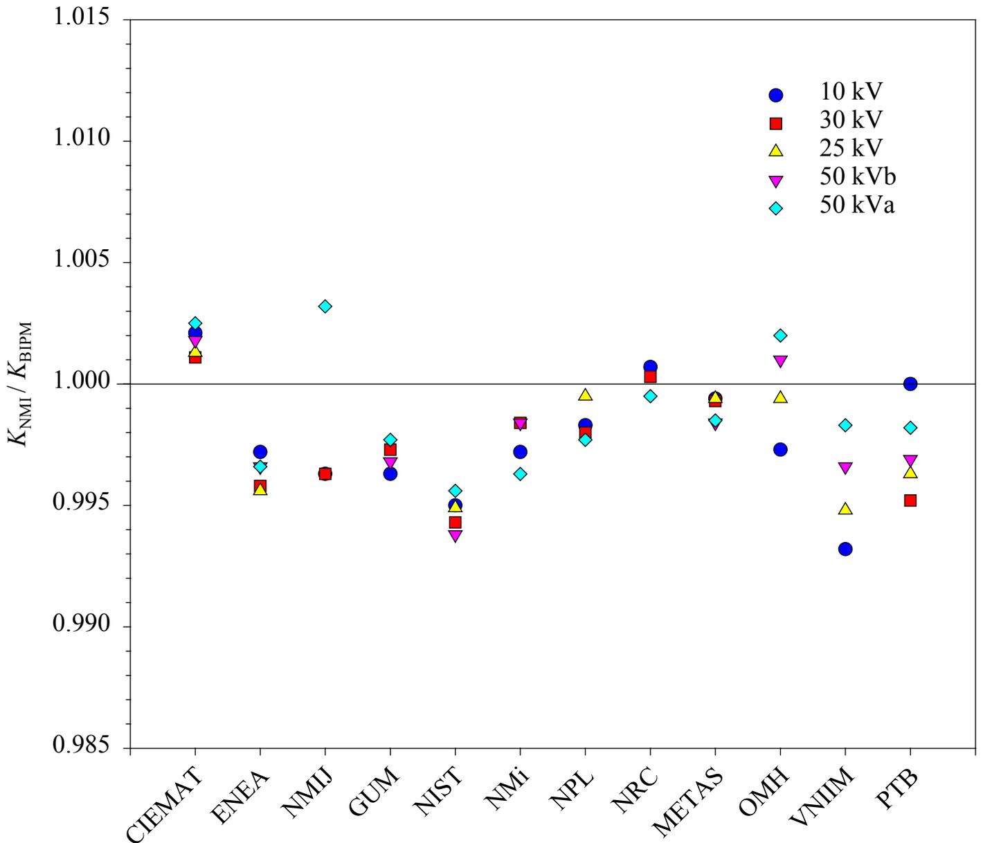
Figure 1. Results of BIPM low-energy x-ray comparisons, expressed as the ratio of the air-kerma rate determined by the standard of the national metrology institute (NMI) to that determined by the BIPM standard. For NMIs that have compared more than once at the BIPM, only the results of the most recent comparison are included.
