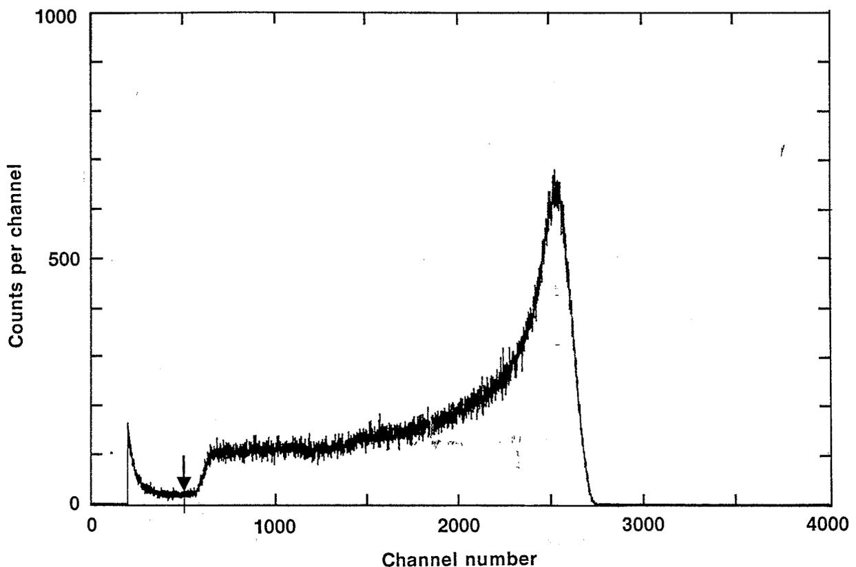
Figure 2. Typical pulse-height spectrum for a Bonner-sphere detector. The discriminator bias at 20 % of the peak is shown by an arrow.
