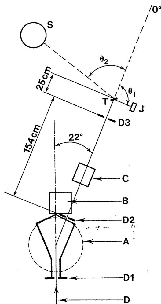
Figure 1. Experimental arrangement for neutron production and fluence measurements. D: deuteron beam; D1, D2, D3: diaphragms; A: magnetic field; B: polyethylene cubic slab shielded with 1 mm Cd; C: electrostatic lens; T: neutron producing target; J: silicon detector,  $\theta_1 = 78^\circ$  at 20 cm for (d+D) neutrons, or  $\theta_1 = 150^\circ$  at 1 m for (d+T) neutrons; S: Bonner sphere,  $\theta_2 = 86^\circ$  and  $26,7^\circ$  for (d+D) and (d+T) neutrons, respectively.
