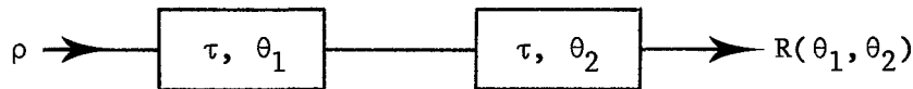
Fig. A1 - Schematic arrangement of two generalized dead times of equal length.
