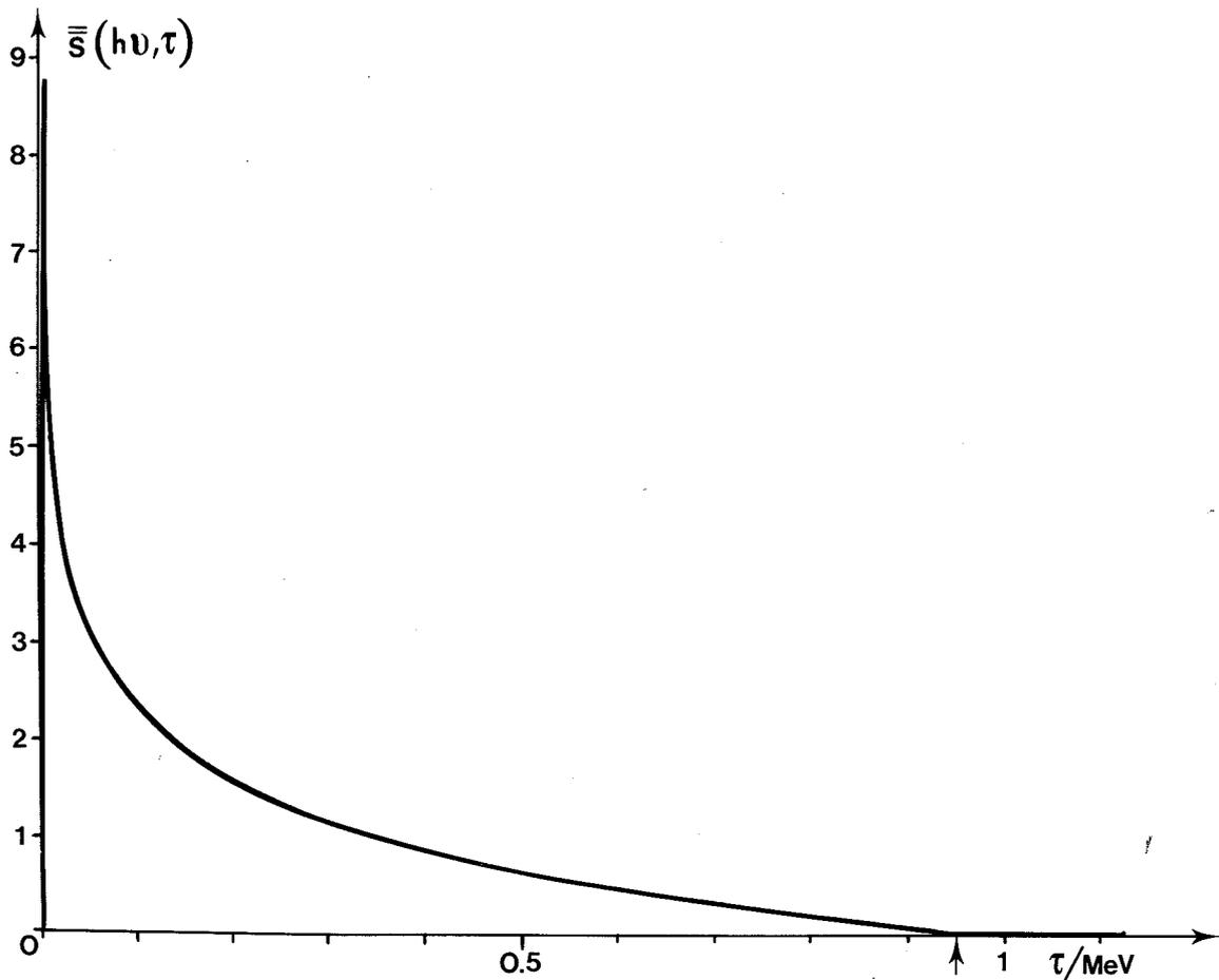
Figure 1 - Spectral distribution  $\bar{S}(h\nu, \tau)$  of the energy fluence of bremsstrahlung photons ( $h\nu = 1.25$  MeV)
