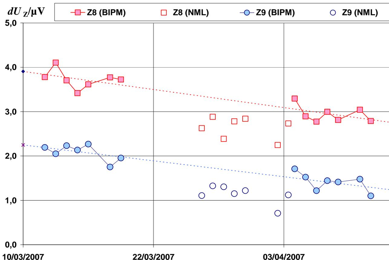
Figure 1. Voltage of BIPM\_8 (Z8) and BIPM\_9 (Z9) at 10 V measured at both institutes, referred to an arbitrary origin, as a function of time, with linear least-squares fit to the measurements of the BIPM.
