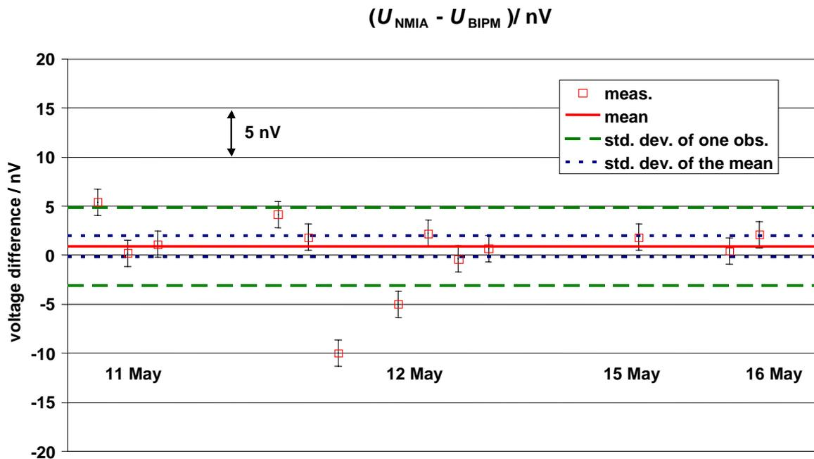
Fig. 1. Differences between the measured values and the theoretical value of the BIPM array voltage. Vertical bars are the mean value of the  $1\sigma$  Type A uncertainties of the measurements (due only to the spread of detector readings during a measurement) and have a value of 1.35nV. The solid lines ( — ) are the  $1\sigma$  Type A uncertainty of the mean, and the dotted lines ( - - - ) are the  $1\sigma$  Type A uncertainty of single measurements.
