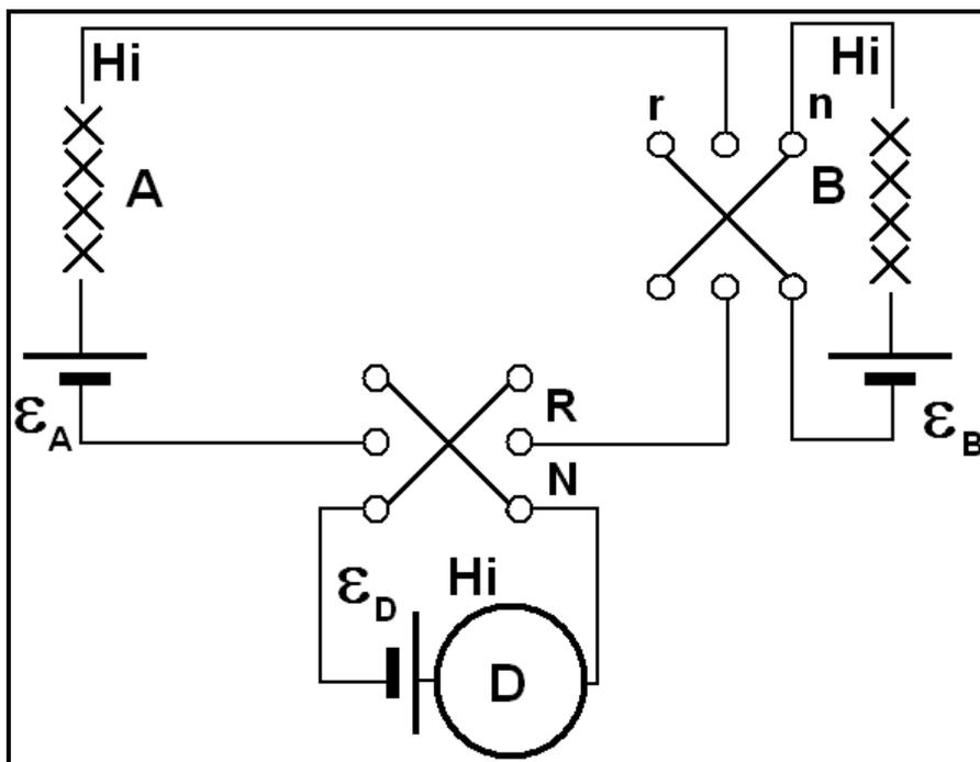
Fig. 2. Schematic diagram of the connections with the detector in normal (N) or reverse (R) position, and with the NMIA array in normal (n) or reverse (r) position. During the Josephson comparison, the NMIA array was always connected in the normal position.
