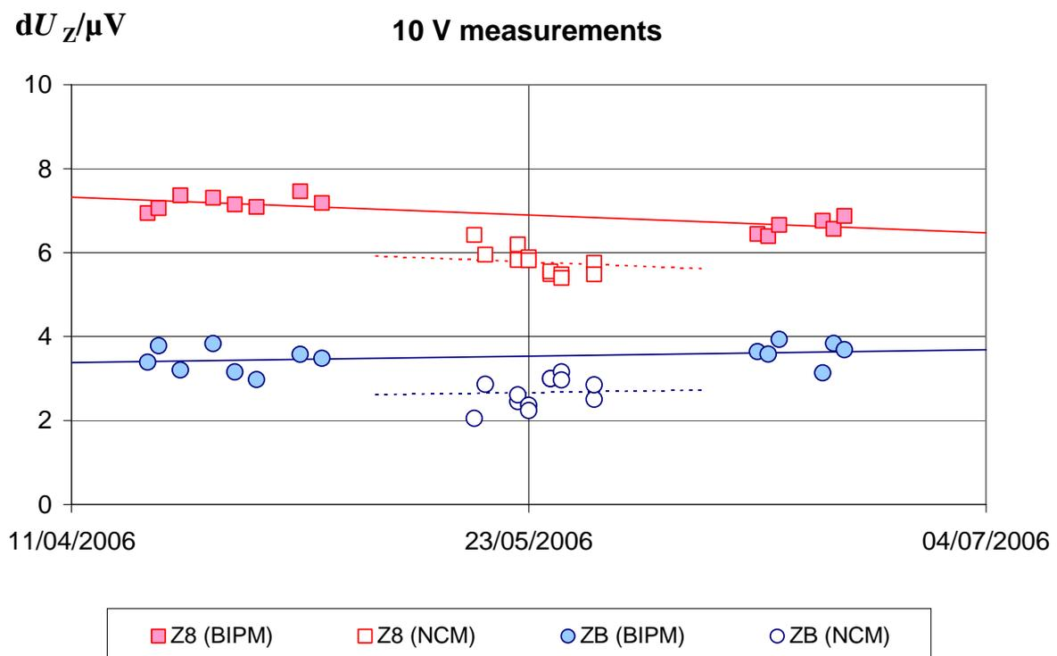
Figure 1. Voltage of Z8 and ZB at 1.018 V and 10 V as a function of time, with arbitrary voltage origins, marked with linear least-squares fits to the measurements of the BIPM.
