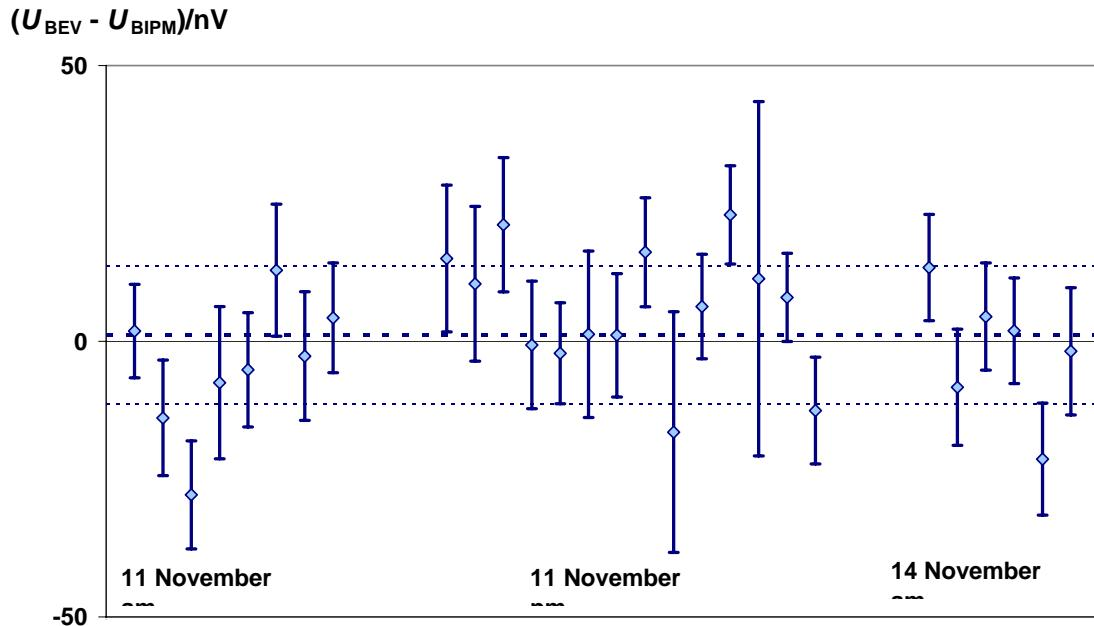
Fig. 1. Difference between the measured values and the theoretical value of the BIPM array voltage. Vertical bars are the  $1\sigma$  Type A uncertainties of each measurement. The dotted lines are for the mean and the  $1\sigma$  Type A uncertainties of a single measurement.
