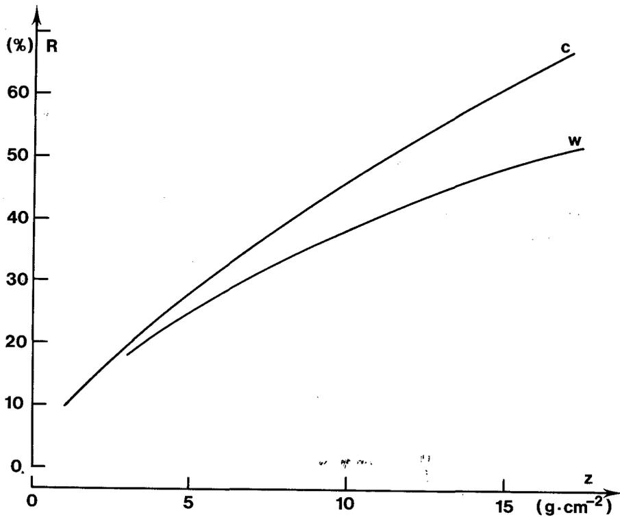
Figure 1 -  $R$  as a function of depth, for a graphite phantom (c) and a water phantom (w), for the BIPM  $^{60}\text{Co}$  beam
