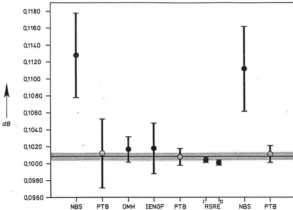
Fig. 12 Measurement results for transfer standard NBS-0.1 (0.1 dB)
