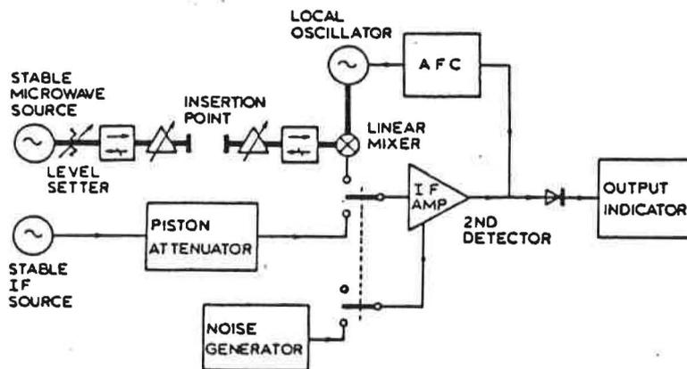
Fig. 8 Simplified circuit diagram of the IF parallel substitution method, applied e.g. at IEN (drawn from WARNER [3])
