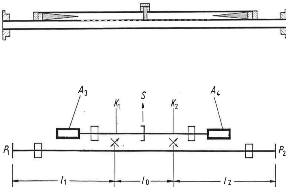
Fig.3 Construction scheme (a) and circuit diagram (b) of the transfer standard PTB-2.22-481 (0.01 dB)  $P_1, P_2$  Input and output port,  $K_1, K_2$  coupling holes,  $A_3, A_4$  matched loads,  $S$  movable short
