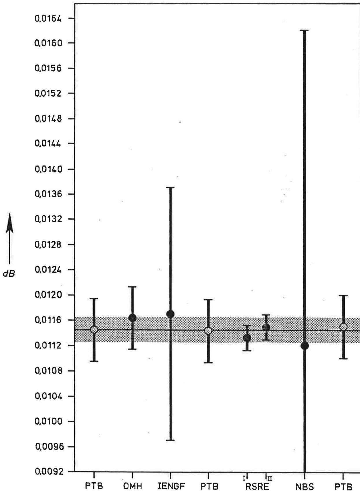
Fig. 11 Measurement results for transfer standard PTB 2.22-481 (0.01 dB)
