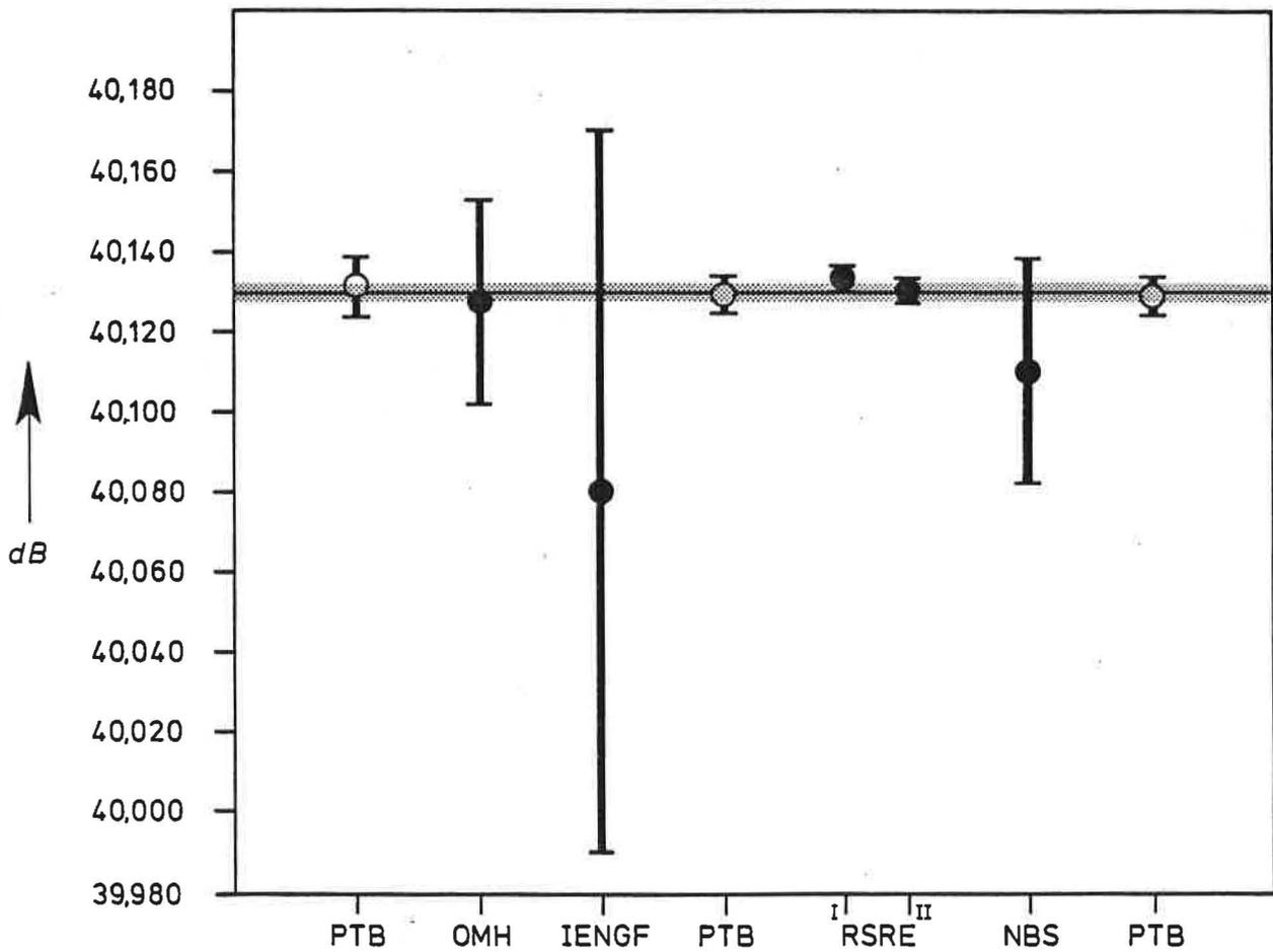
Fig. 15 Measurement results for the transfer standard PTB-2.22-311 (40 dB)
