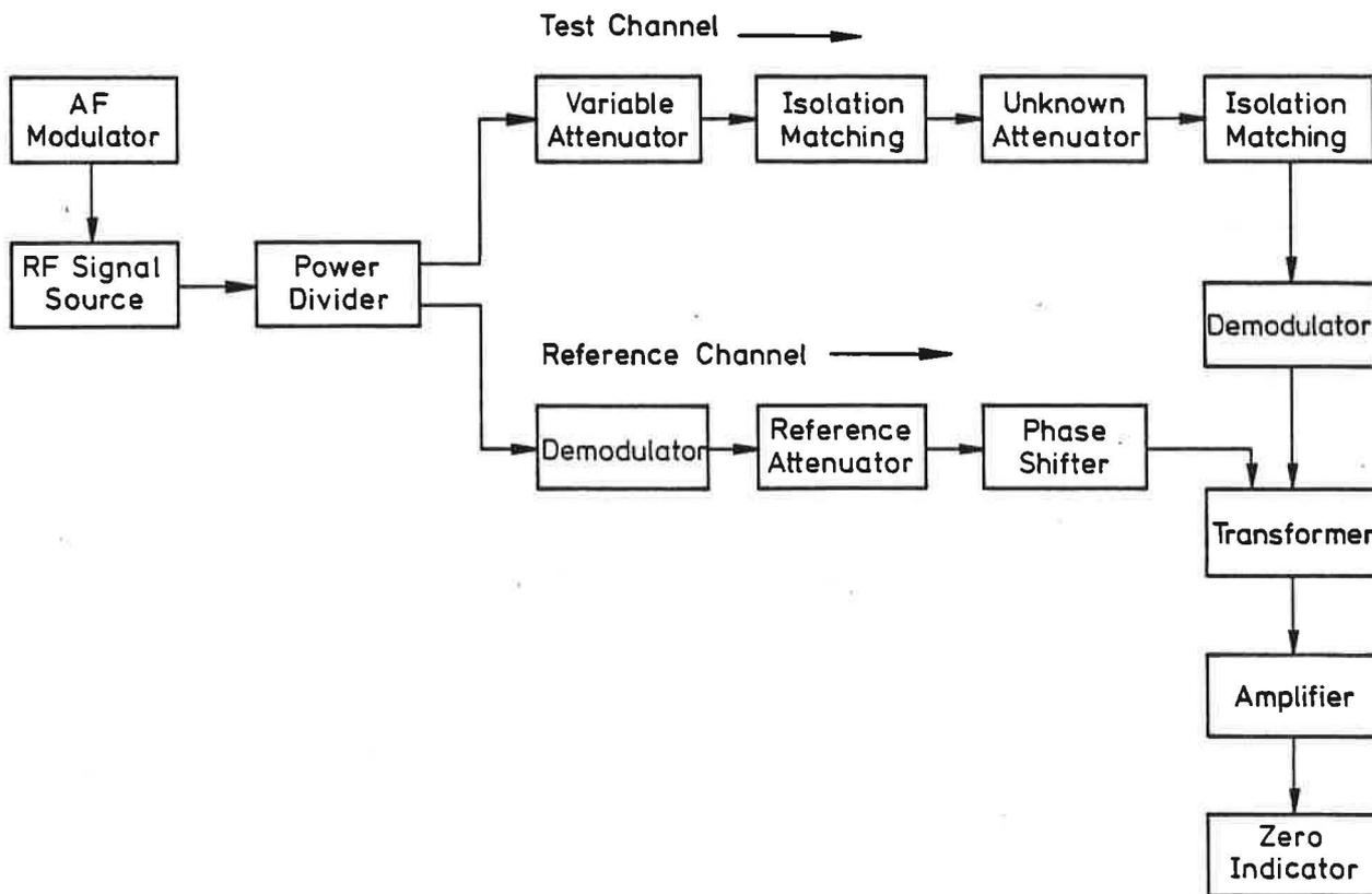
Fig. 6 Block diagram of the audio frequency substitution method as applied at OMH. The transformer is an inductive voltage divider (IVD)
