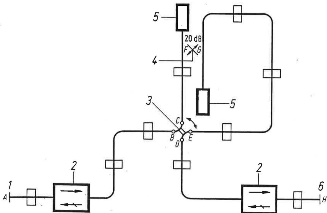
Fig. 4 Circuit diagram for transfer standard PTB-2.22-311 (40 dB)
