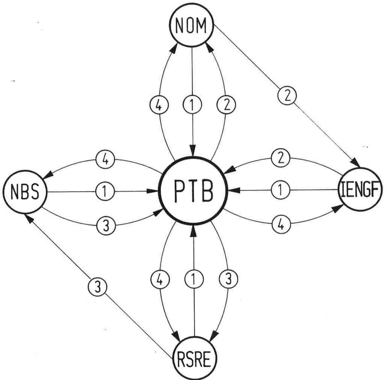
Fig 1 Intercomparison pattern for the international intercomparison GT-RF 75-A 3 (Attenuation in waveguide R 140 at 15 GHz)
