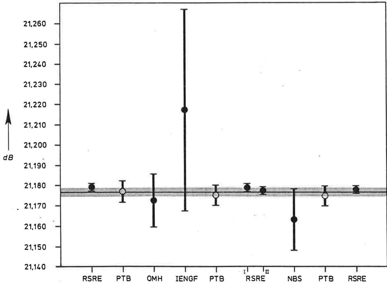
Fig. 14 Measurement results for transfer standard UK-18-S2 (20 dB)
