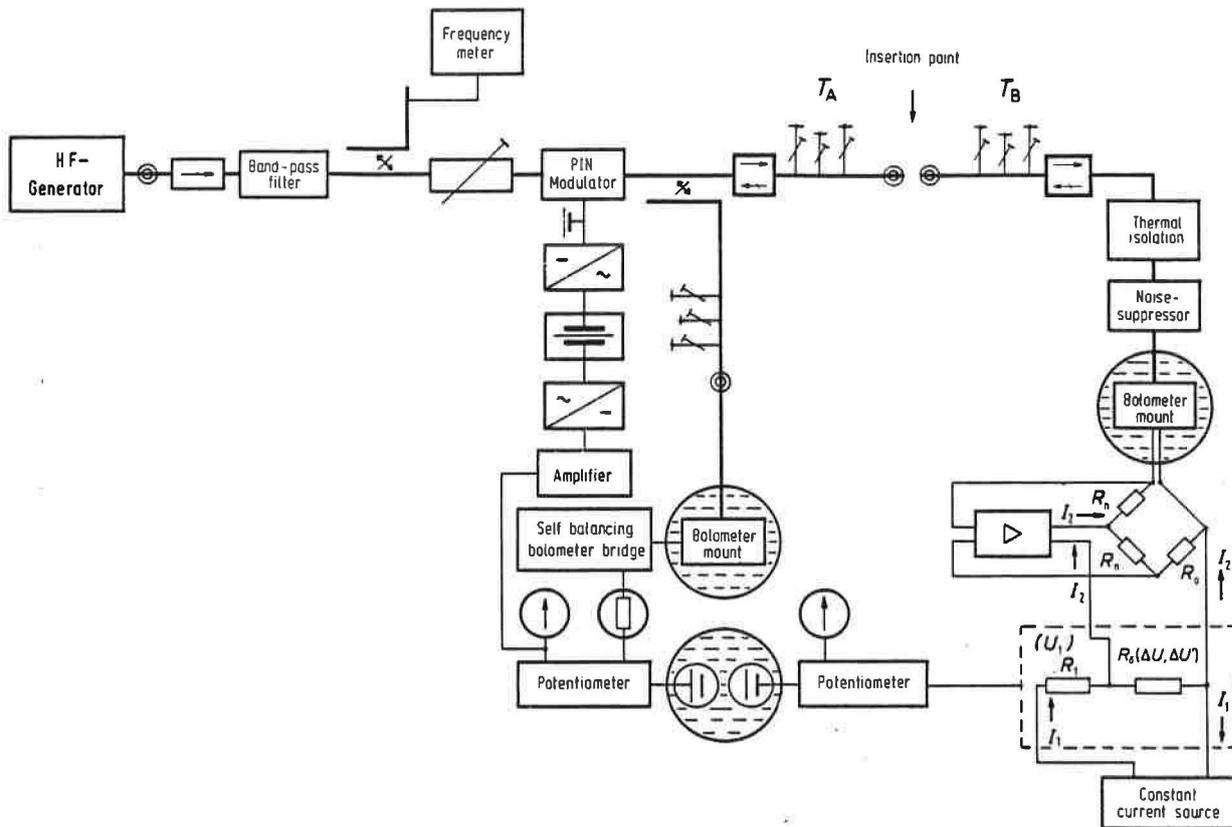
Fig. 5 Circuit diagram of the power ratio measuring equipment as established at PTB
