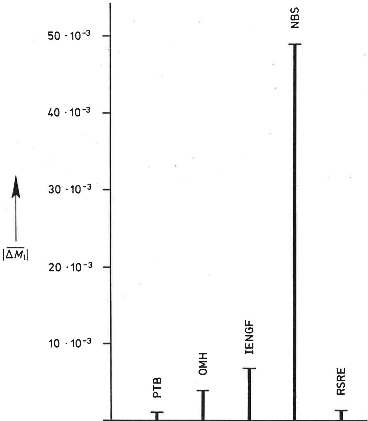
Fig. 16 Mean values averaged over the magnitudes of all relative deviations from the weighted mean values of all five transfer standards; given for each participating laboratory
