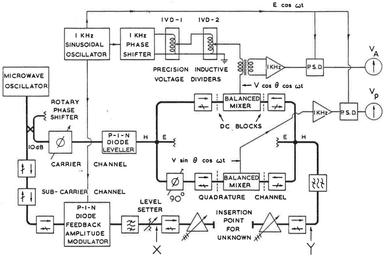
Fig.7 Circuit diagram of the modulated subcarrier technique as established at RSRE (drawn from WARNER, HERMAN and JEFFS)
