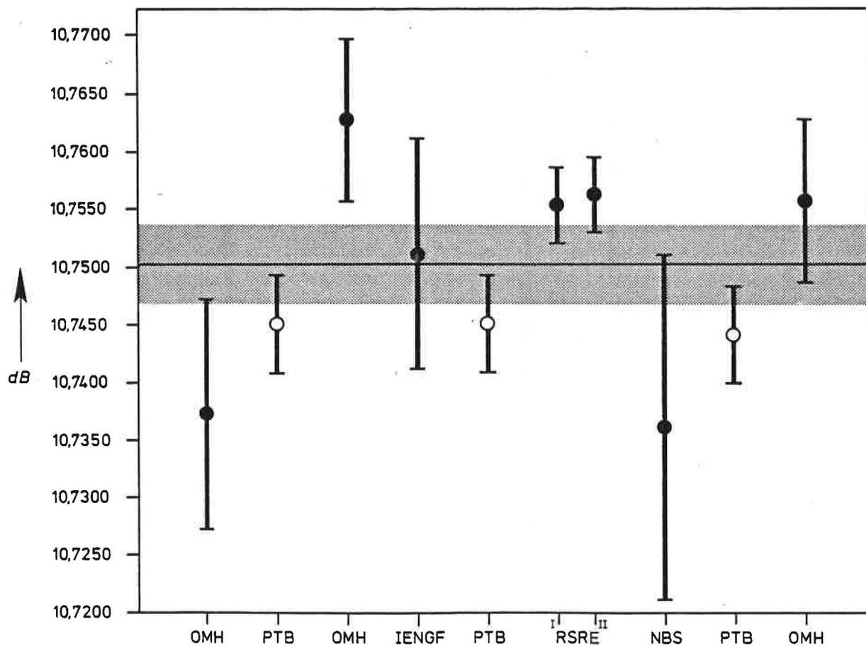
Fig. 13 Measurement results for transfer standard OMH-10-01 (10 dB)
