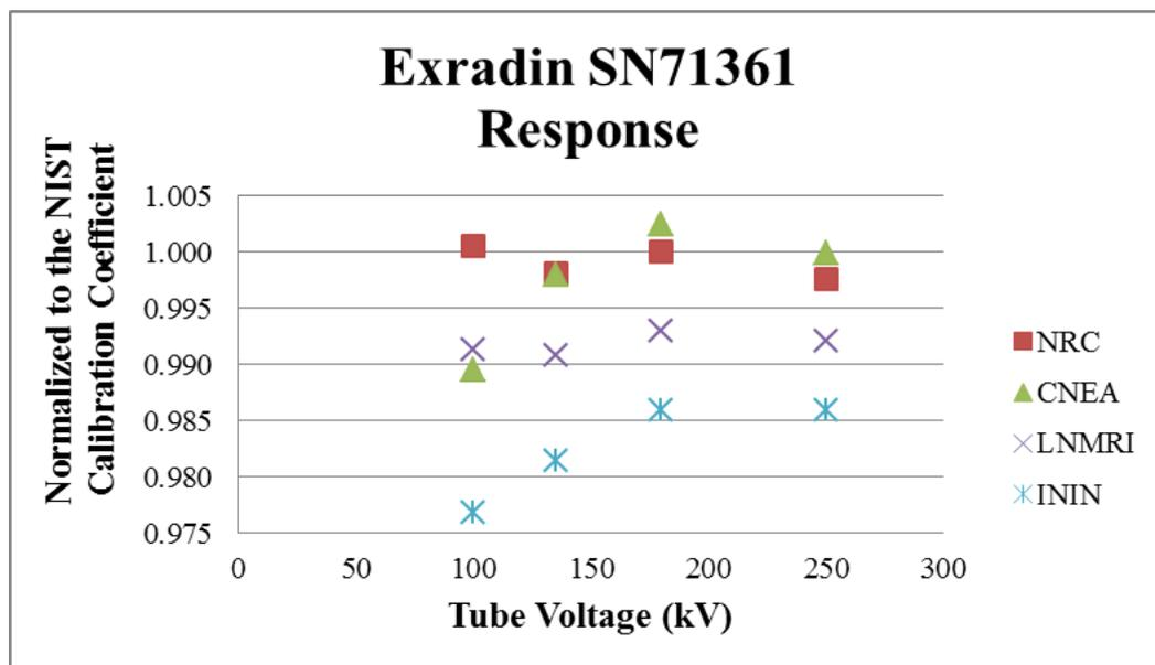
**Figure 3.** Relative calibration coefficients measured with the Exradin SN 71361 as a function of the tube voltage, normalized to the NIST average, as shown in Table 15.
