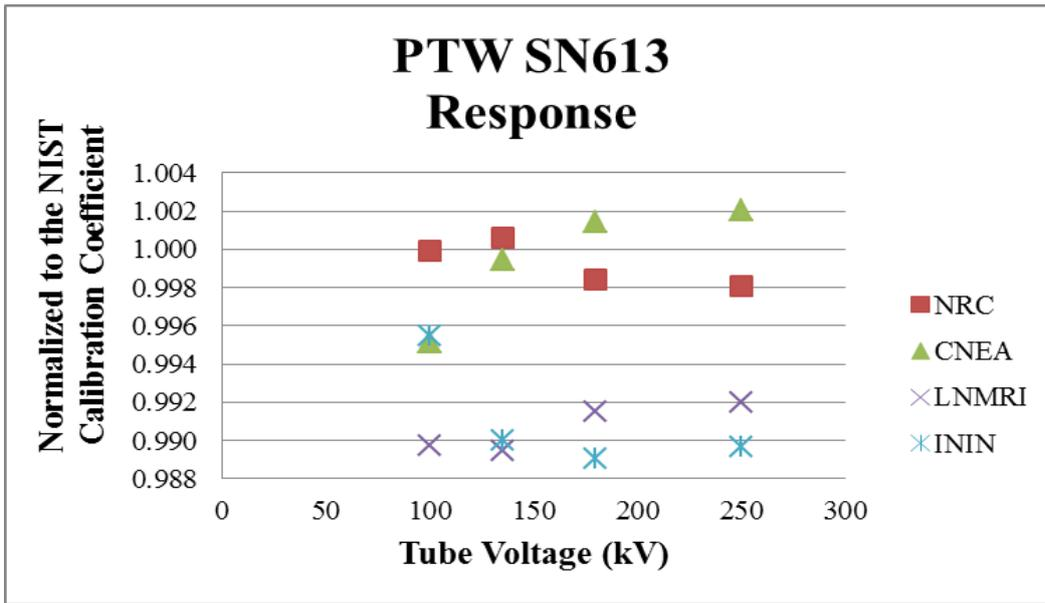
**Figure 1.** Relative calibration coefficients measured with the PTW SN613 for all participants as a function of the tube voltage, normalized to the NIST average, as shown in Table 15.
