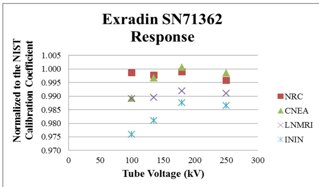
**Figure 4.** Relative calibration coefficients measured with the Exradin SN 71362 as a function of the tube voltage, normalized to the NIST average, as shown in Table 15.
