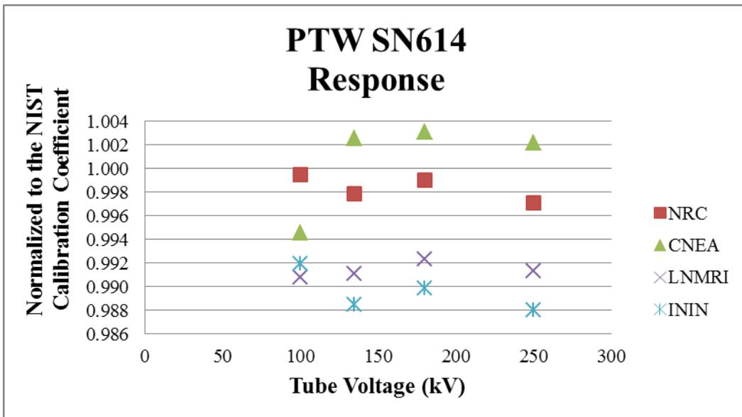
**Figure 2.** Relative calibration coefficients measured with the PTW SN614 as a function of the tube voltage, normalized to the NIST average, as shown in Table 15.
