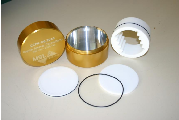
Figure 2. Anodized Aluminium/Teflon containers for transportation and storage of filters.
