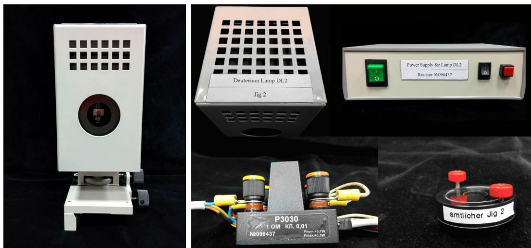
Figure 3.1. Measurement artifact: deuterium lamp in housing, power supply, shunt resistor and alignment jig
