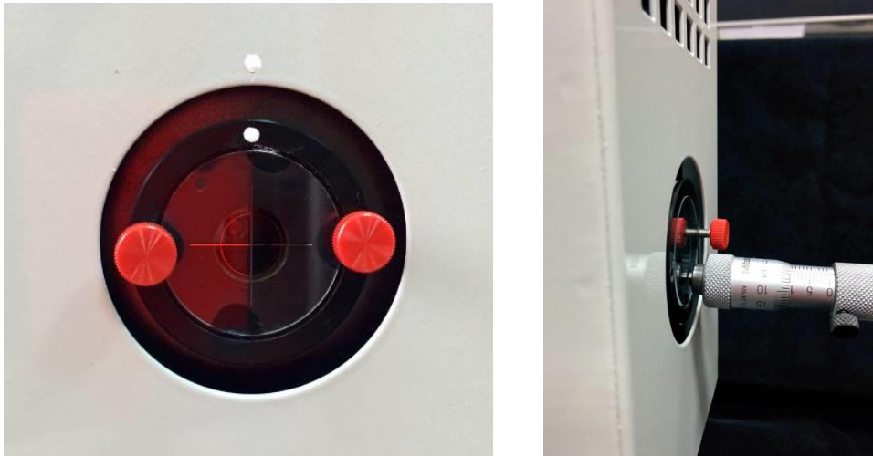
Figure 3.2. Alignment jig (right) and reference plane for the distance measurement (left)
