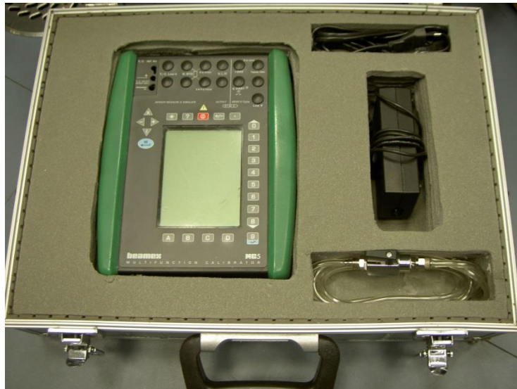
Figure 3 The transfer standard, battery charger and tubing with valve
