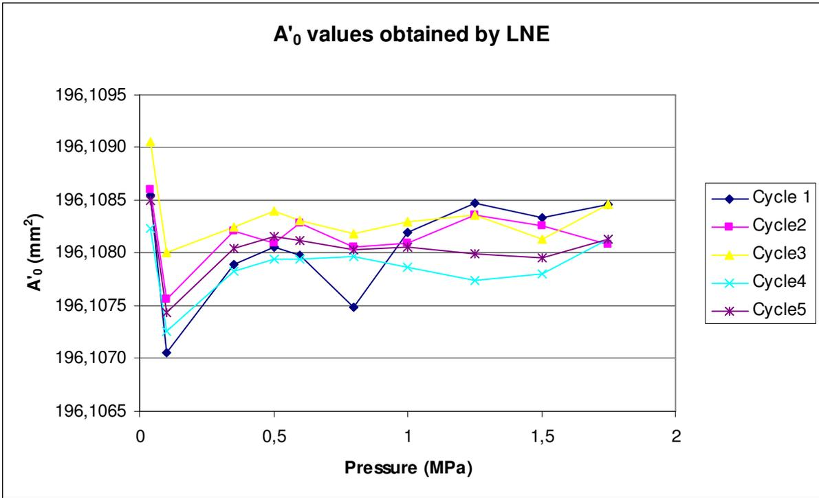
Figure 1- Effective area values against the pressure for each cycle (LNE)
