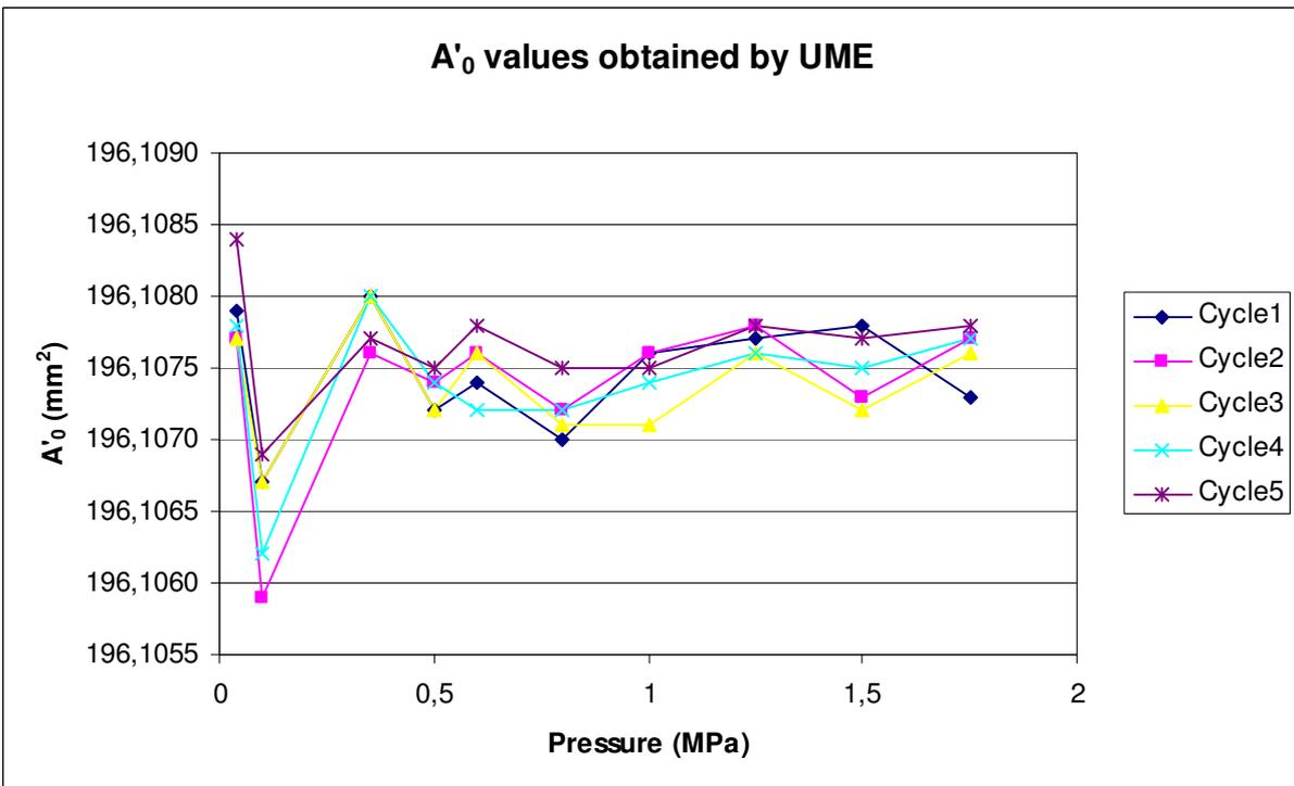
Figure 2- Effective area values against the pressure for each cycle (UME)
