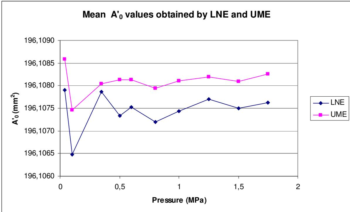
Figure 3 - Mean effective area values vs pressure for each cycle obtained by LNE and UME
