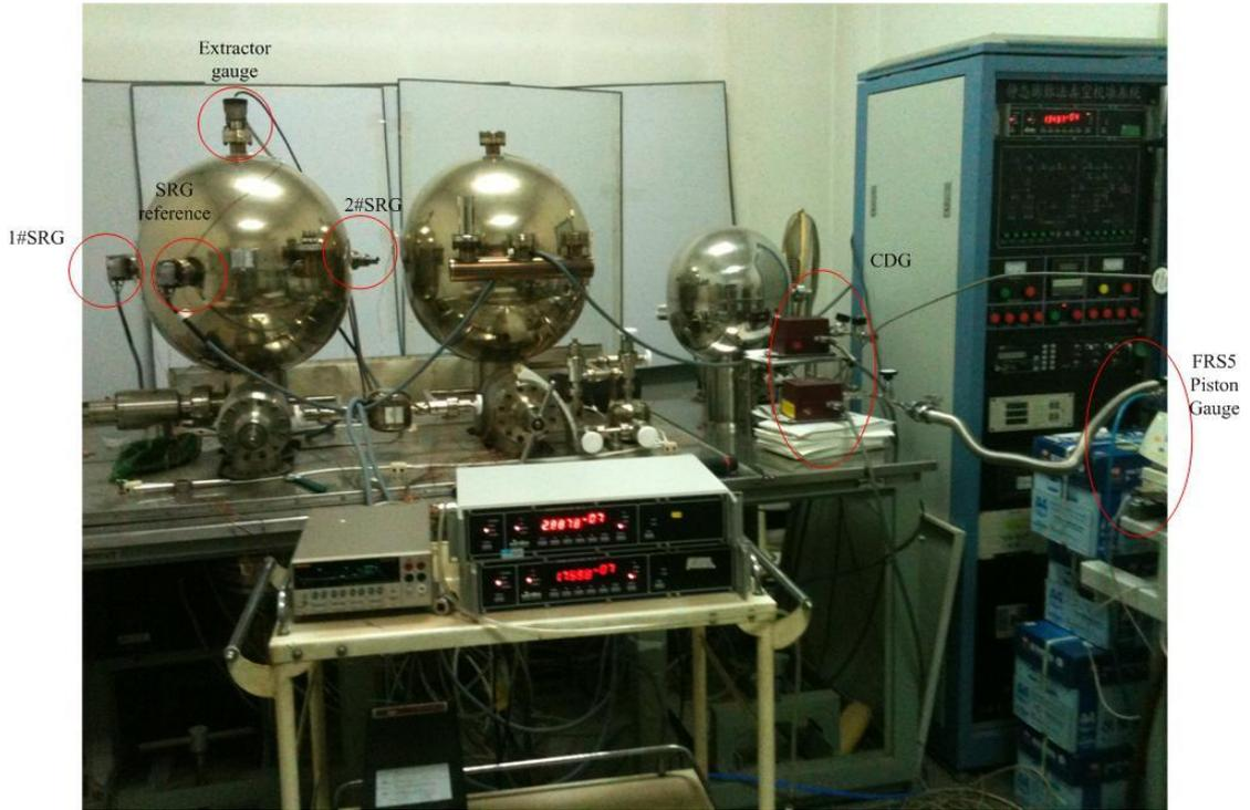
**Fig. 2:** Picture of the expansion system
