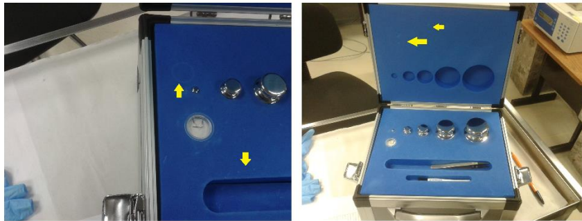
Image 5. Apparent damage inside the transportation box after circulation
