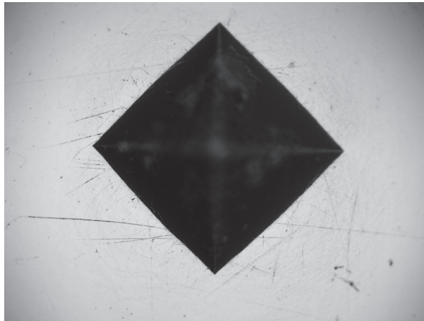
Fig. 3.6 Reference indentation of 200 HV 30 observed with 20× objective lens (NA=0.40).
