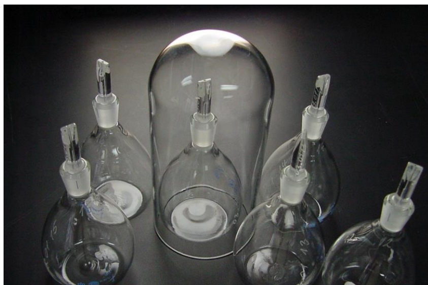
Figure 7. An image of the Gay-Lussac type pycnometers for volumes of 100 mL.
