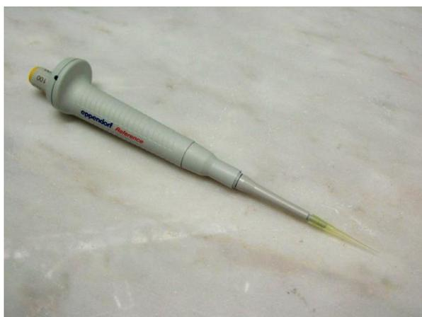
Figure 1. Fixed micropipette of 100  $\mu\text{L}$
