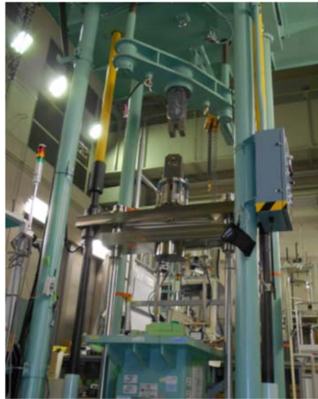
Fig. 1. The NMIJ's 100 kN DWM.
