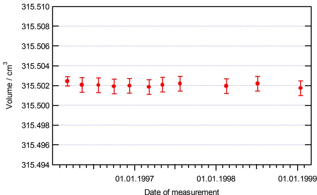
Fig. 2: Monitoring at OFMET, results and uncertainty bars ( $k=2$ ) for the volume of the sphere CS 85 as a function of the date of measurement. The scale is deliberately the same as in Fig. 4.
