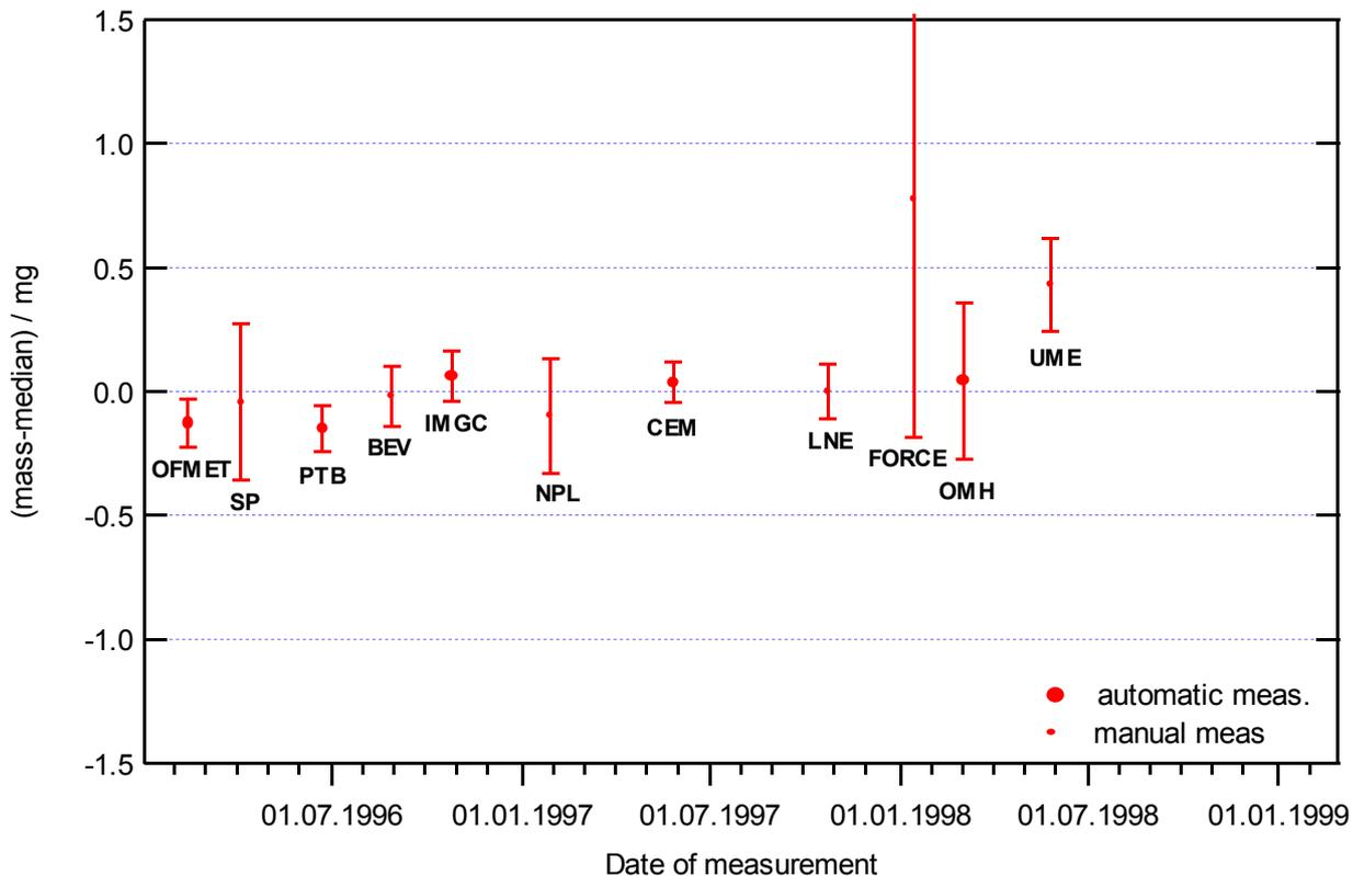
Fig. 15: Mass of the sphere CS 55, deviation with respect to the median and associated expanded uncertainty ( $k=2$ ).
