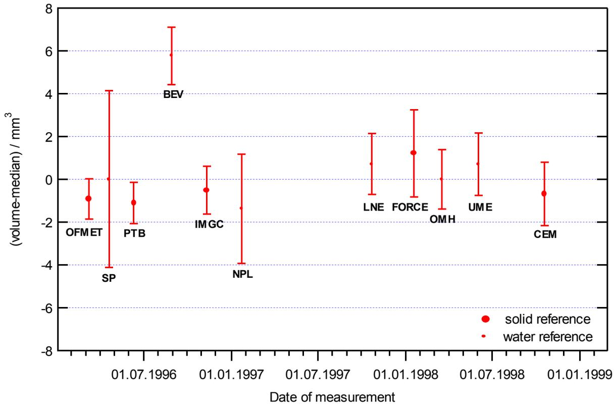
Fig. 11: Volume of the sphere CS 75, deviation with respect to the median and associated expanded uncertainty (k=2)
