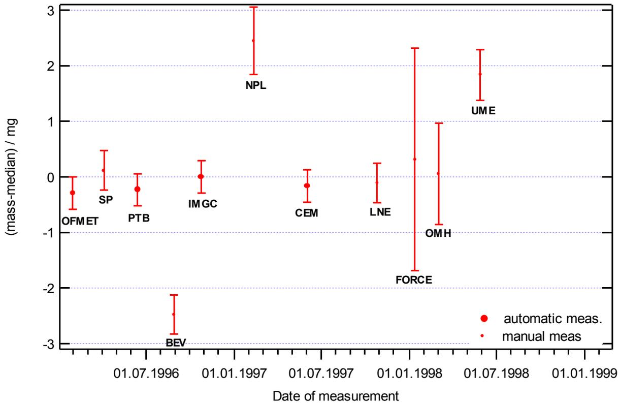
Fig. 13: Mass of the sphere CS 85, deviation with respect to the median and associated expanded uncertainty (k=2).
