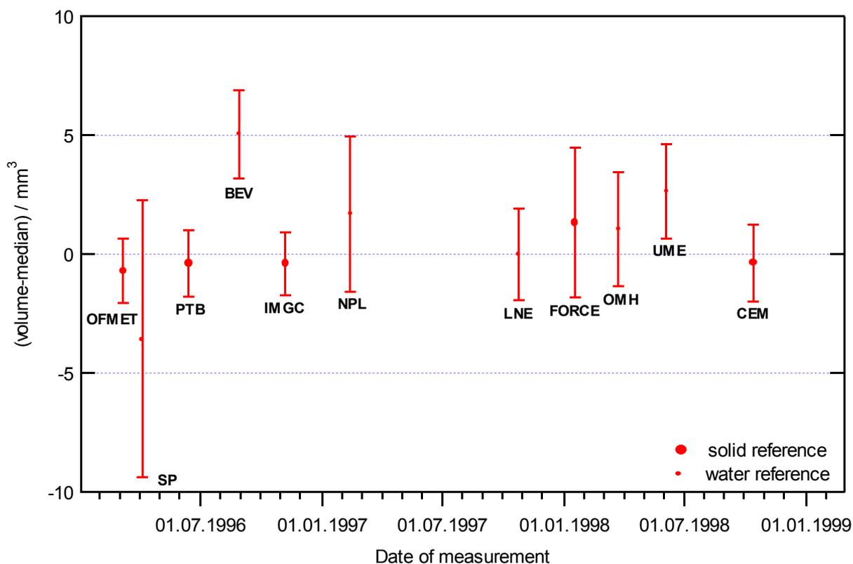
Fig. 10: Volume of the sphere CS 85, deviation with respect to the median and associated expanded uncertainty (k=2).
