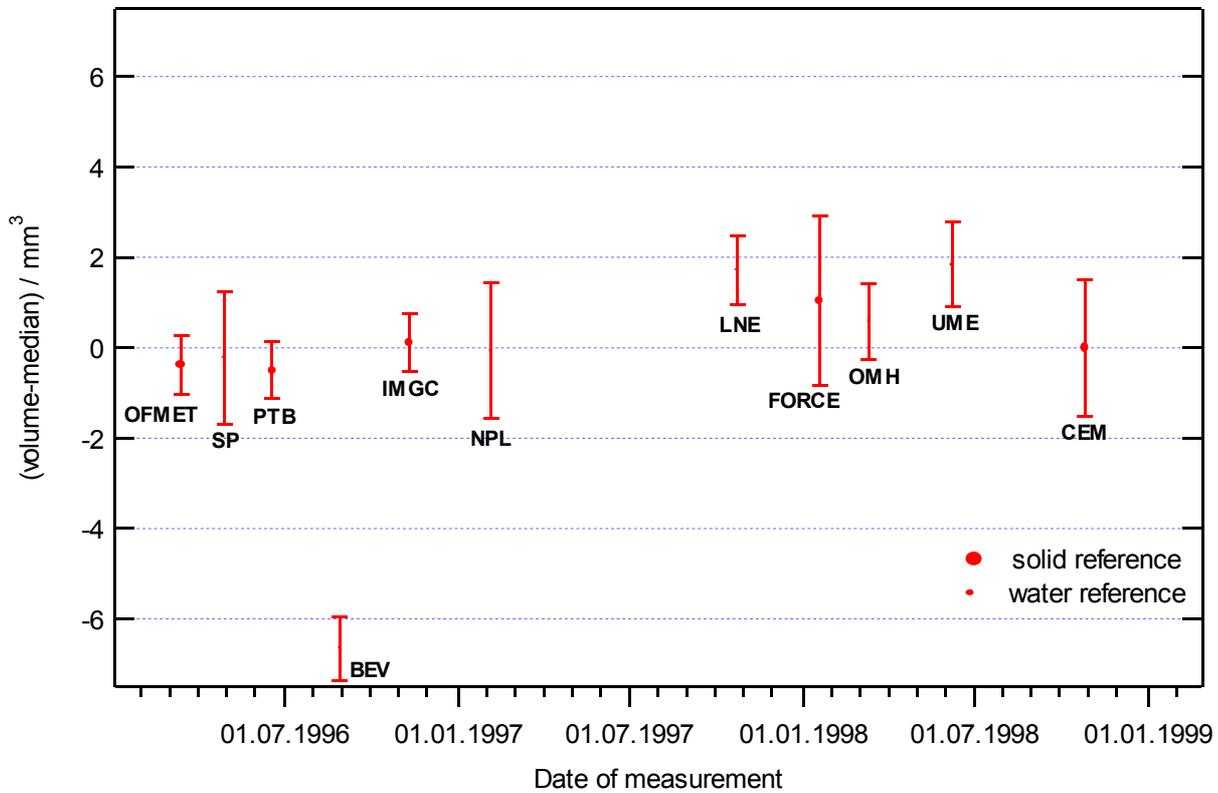
Fig. 12: Volume of the sphere CS 55, deviation with respect to the median and associated expanded uncertainty (k=2).
