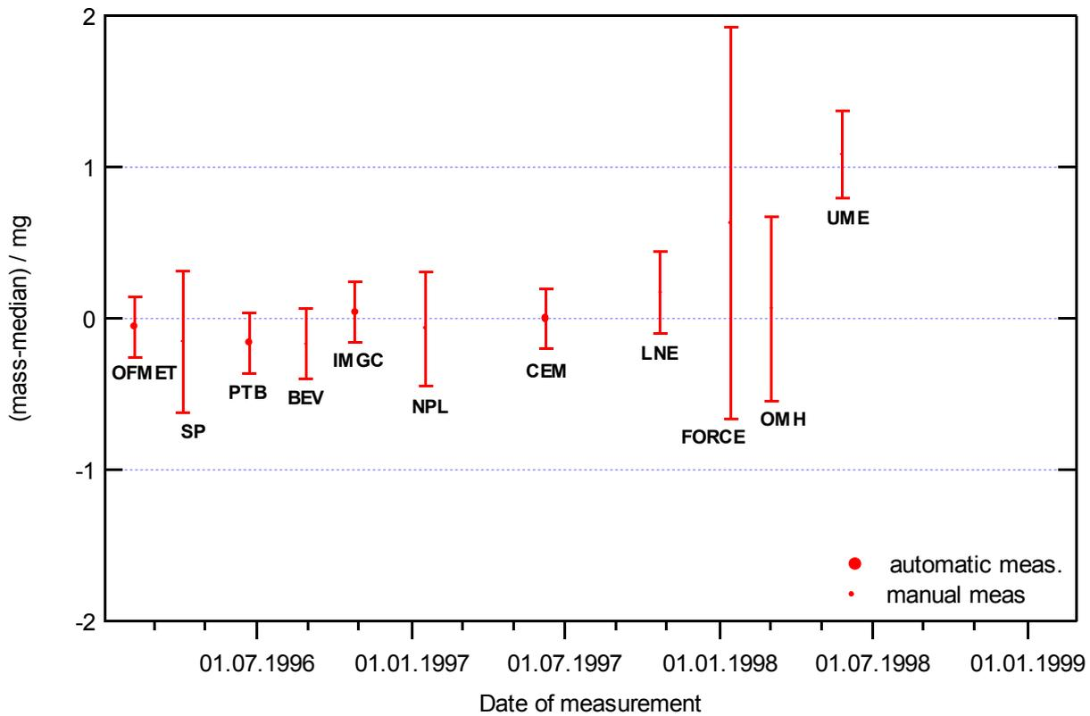
Fig. 14: Mass of the sphere CS 75, deviation with respect to the median and associated expanded uncertainty (k=2).
