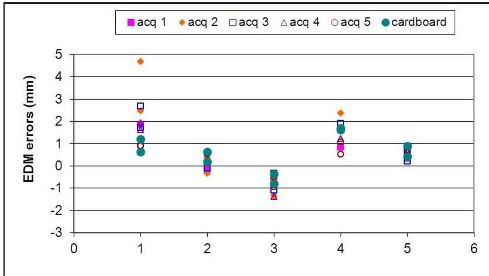
Fig. 13: EDM errors at 20 m (1=DISTO D3a, 2= DLE 150, 3 = GLM 150, 4= DLE 50, 5 = DISTO D8)
