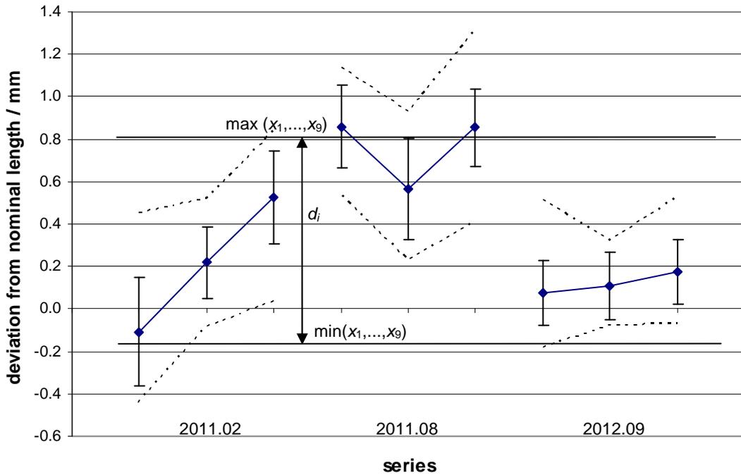
Fig. 4. Results of all series of measurements for Leica DISTO D8 for a distance of 10 m.
