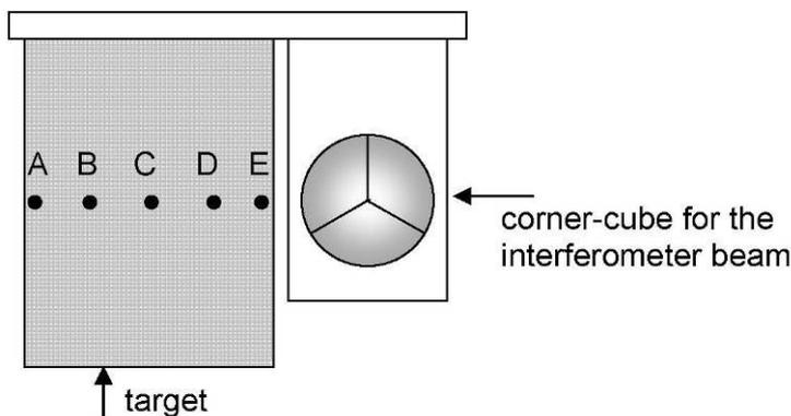
Fig. 11: positions of the laser spot on the target to study the dependence of the EDM errors on the laser spot position (front view)
