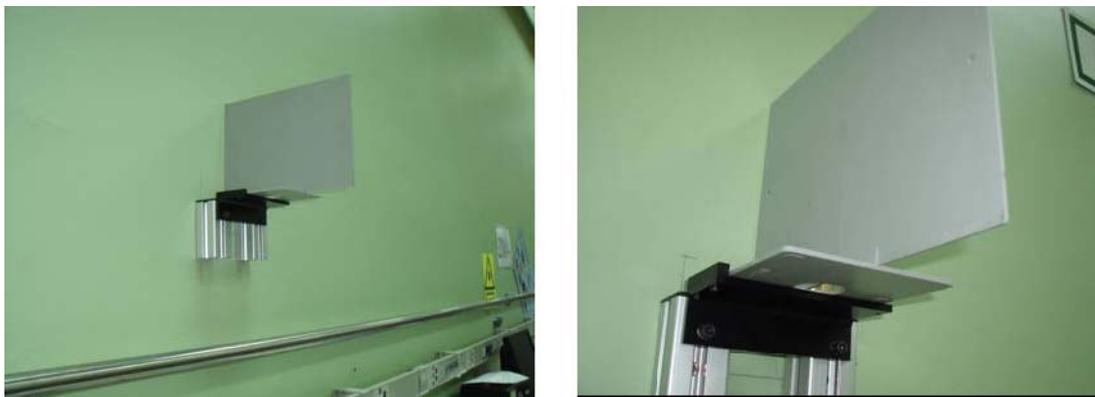
Fig. 3 - View of the comparison target on one of the supports of the baseline (left). A closer look showing the target edge against the support rigid reference (right)
