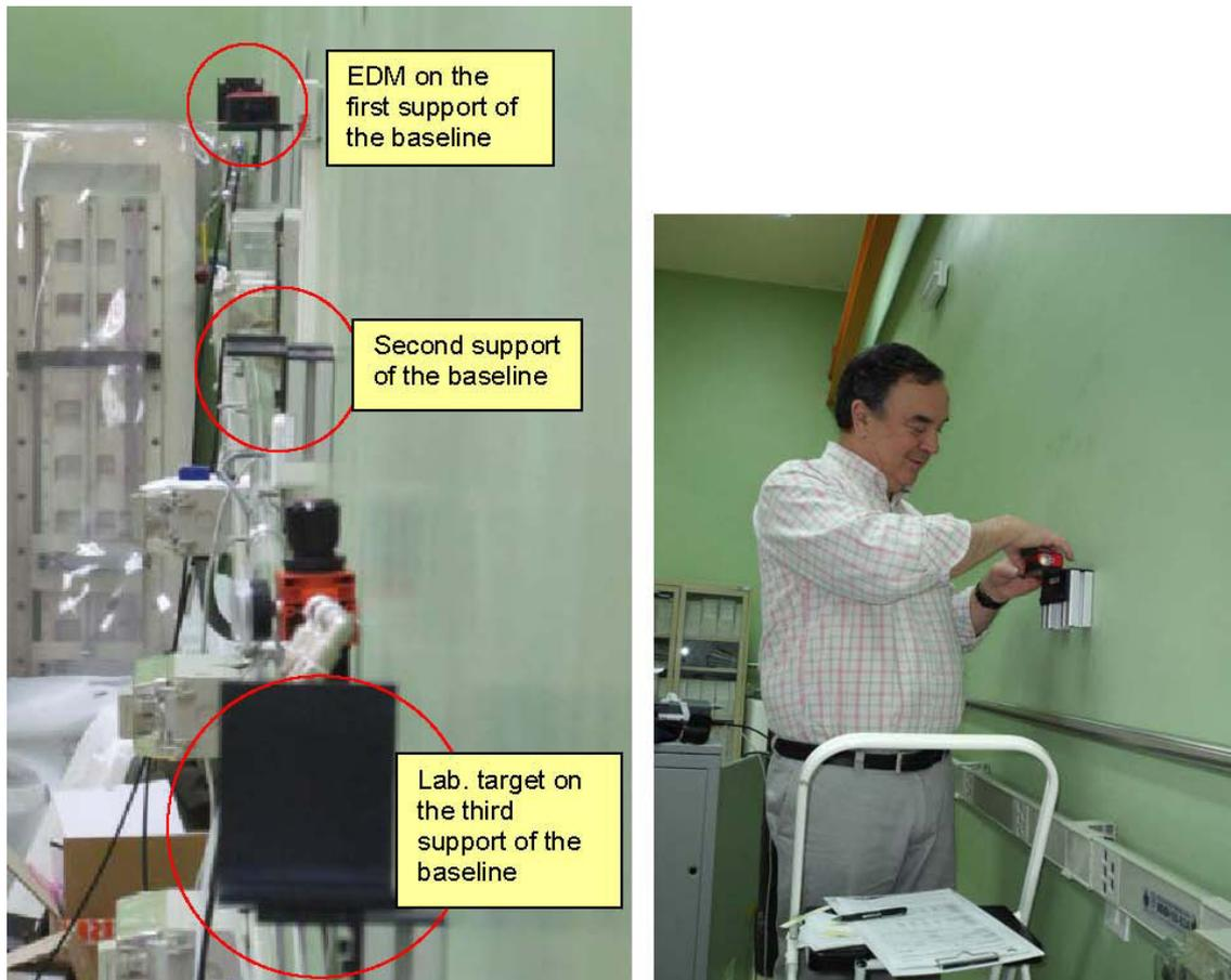
Fig. 1 - View of three consecutive supports of the 50 m baseline (left). Lab. technician situating an EDM on the first support of the baseline (right)
