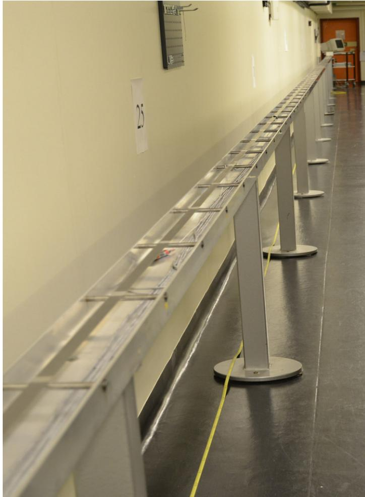
The bench consists of a simple aluminium U-shaped profile with polished steel pins acting as supports for the tape. The bench is a little over 50 m long, and works as support for the reference tape and the calibrated EDMs simultaneously.
