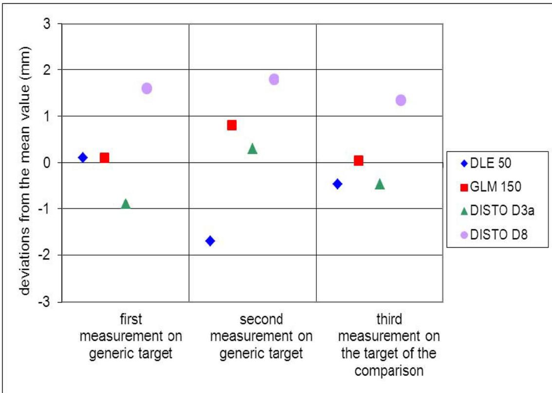
Fig. 15: Deviations from average value of the measurements At 50 m.
