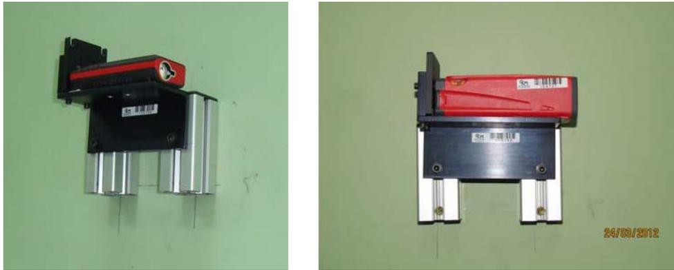
Fig. 2 - View of an EDM on the first support of the baseline (left). A closer look showing the support adjustments and the origin plate (right)
