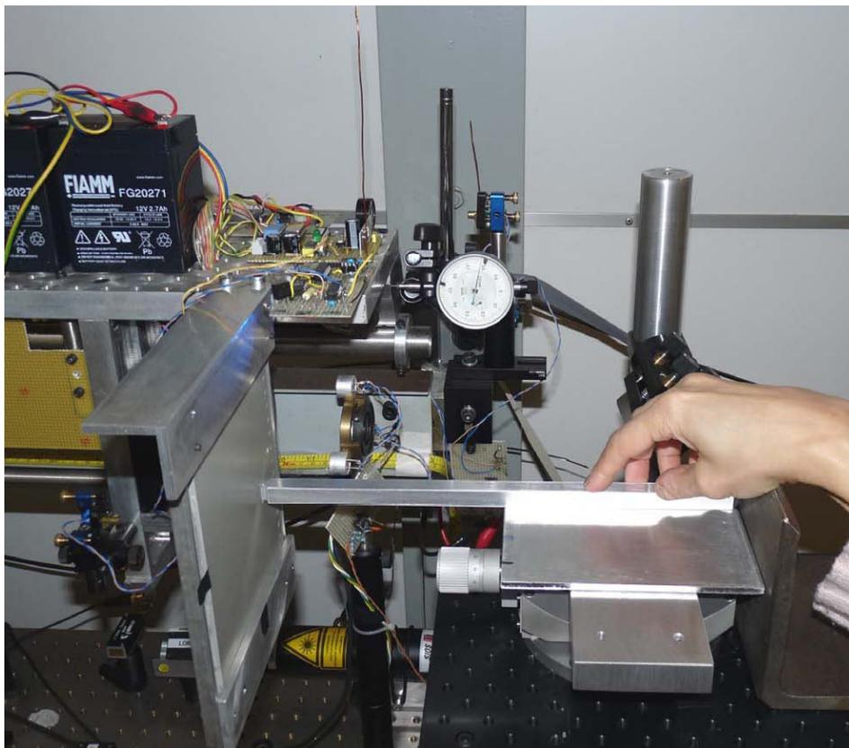
Fig. 6: measurement of the first 30 cm: the ruler touching the stop-wall and the target and the mechanical probe (in the back) touching the carriage are visible.
