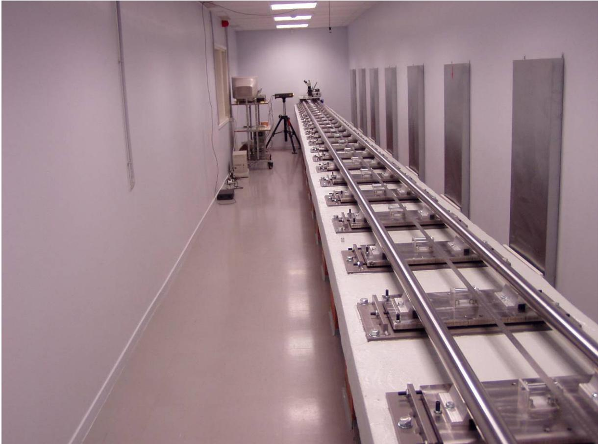
The 21-m bench is located in the designated corridor-like laboratory room. The lab is air-conditioned and the stability of temperature is typically  $\pm 0,5$  °C. There are three humidity and temperature sensors in room for stability and gradient monitoring.
