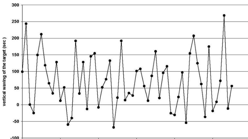
Fig. 9: vertical waving of the target measured by an electronic level placed on the carriage
