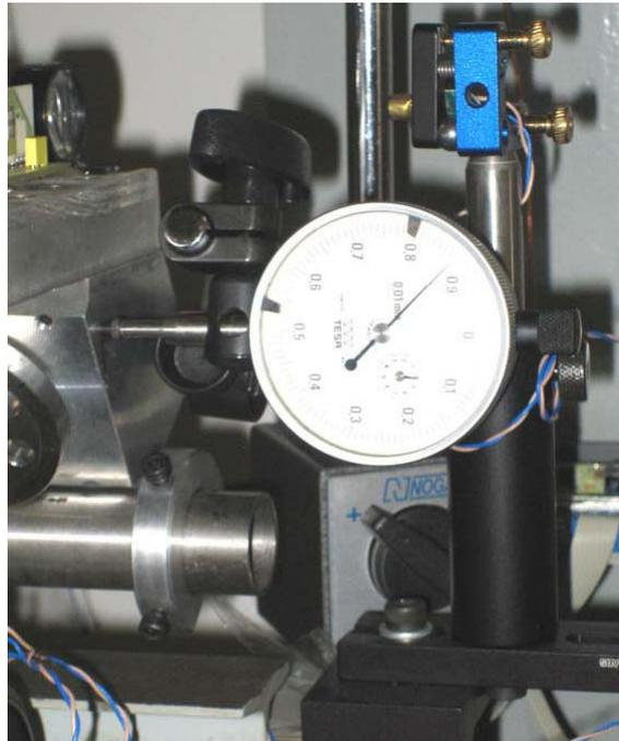
Fig. 7: detail of the mechanical probe touching the carriage
