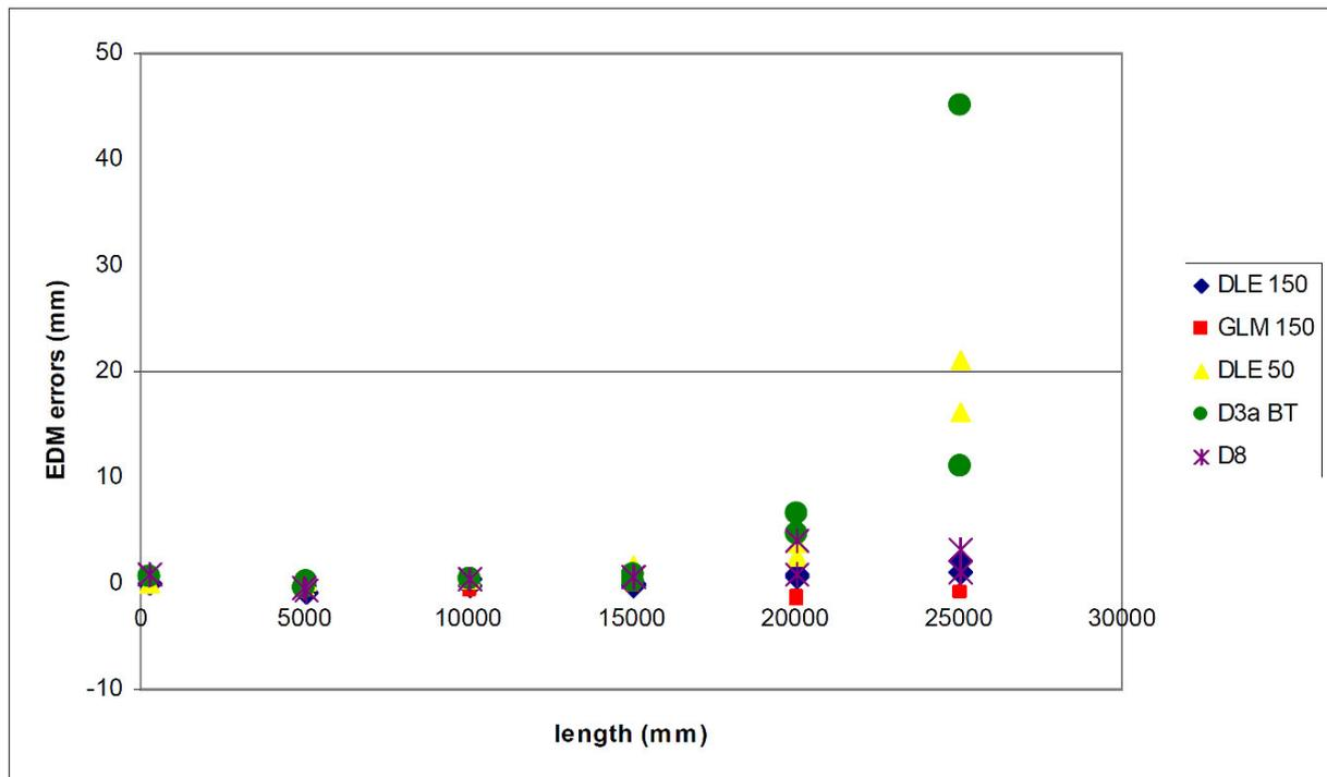
Fig. 10: errors of each EDM in a preliminary set of measurements
