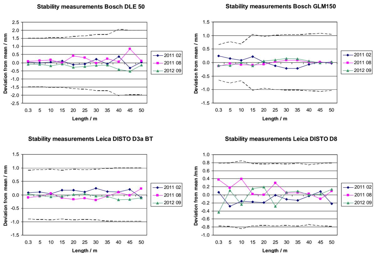
Fig. 1. Measurements of the pilot laboratory monitoring the stability of all four EDMs at each of the measuring distances, bounded by the expanded measurements uncertainty (for  $k=2$ ; dashed line). The solid curves represent deviation from the arithmetic mean of the three measurements.
