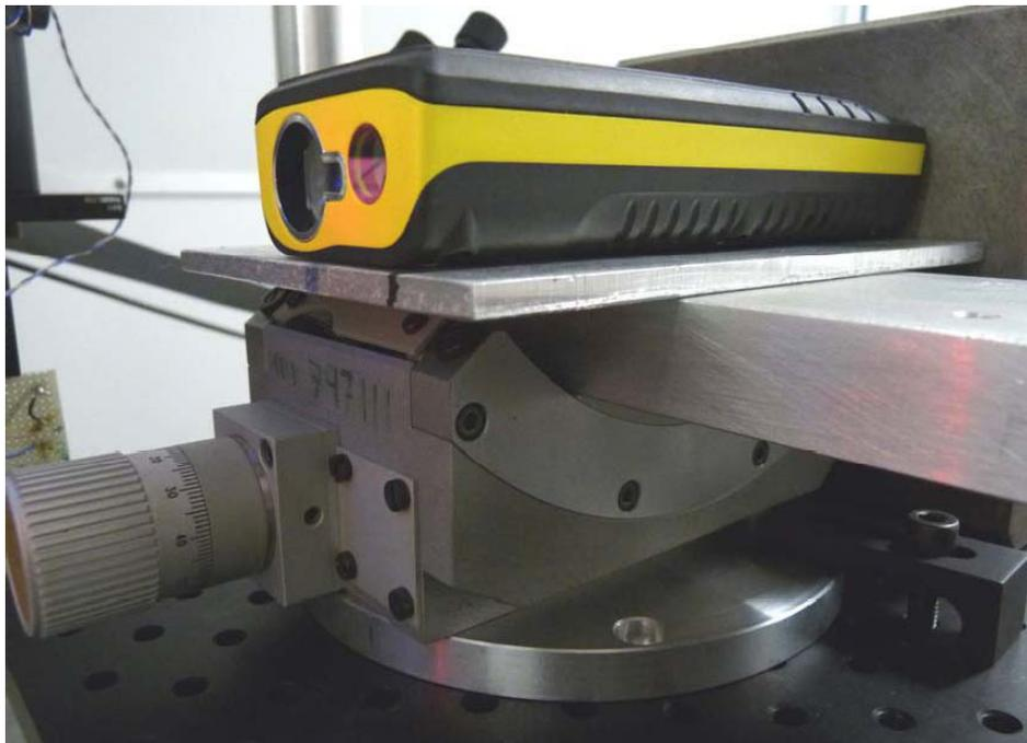
Fig. 5: detail of EDMs' positioning: the cradle-like platform and the stop-wall are well visible.
