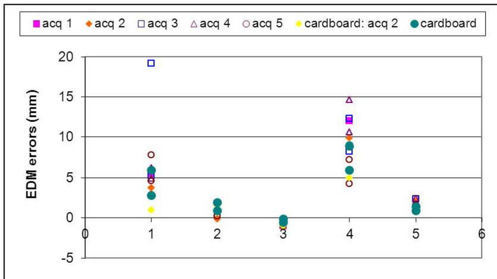
Fig. 14: EDM errors at 25 m (1=DISTO D3a, 2= DLE 150, 3 = GLM 150, 4= DLE 50, 5 = DISTO D8)
