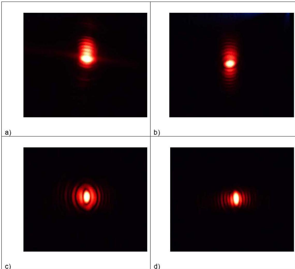
Fig. 12: Laser spot of different EDMs at 25 m: a) Bosch GLM 150, b) Bosch DLE 50, c) Leica DISTO D3a, d) Leica DISTO D8
