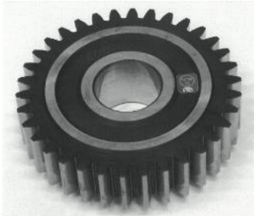
Teilungsnorm, Kennnummer 4693 Pitch measurement standard serial No. 4693
