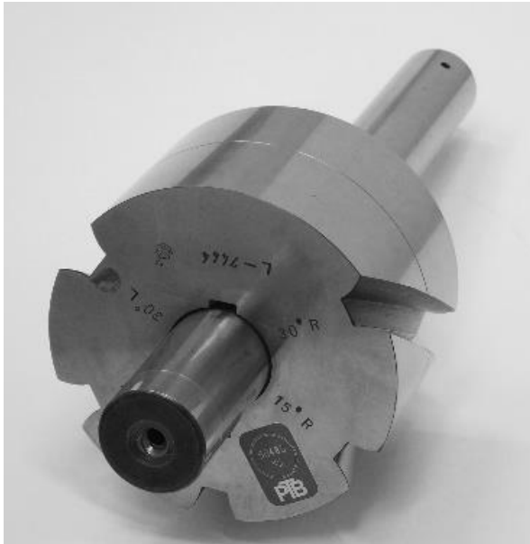
Figure 2: Helix measurement standard (0°, 15°, 30°, left- and right-hand, left flanks)
