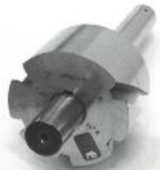
Stirnradnormal Kennnummer Nr. L-7444-1 Cylindrical gear standard serial No. L-7444-1
