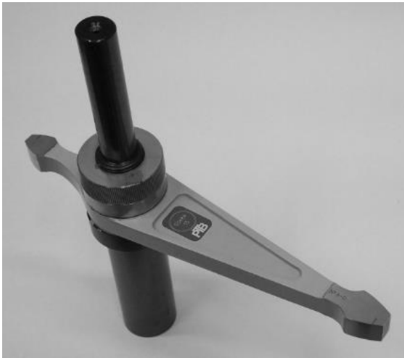
Figure 1: Profile measurement standard (Involute): d_1 = 120 mm and d_2 = 300 mm, right flanks
