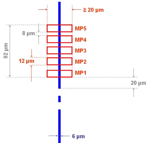
Fig. 2: Locations of the 5 measurement positions (of  $20\ \mu\text{m} \times 12\ \mu\text{m}$  each, with a spacing of  $8\ \mu\text{m}$  between neighbouring MPs). The whole area extends over  $92\ \mu\text{m} \times 20\ \mu\text{m}$ .
