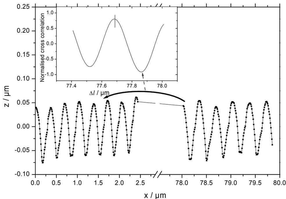
Fig. A2: Illustration of cross correlation analysis for single AFM measurement line of pitch measurement.
