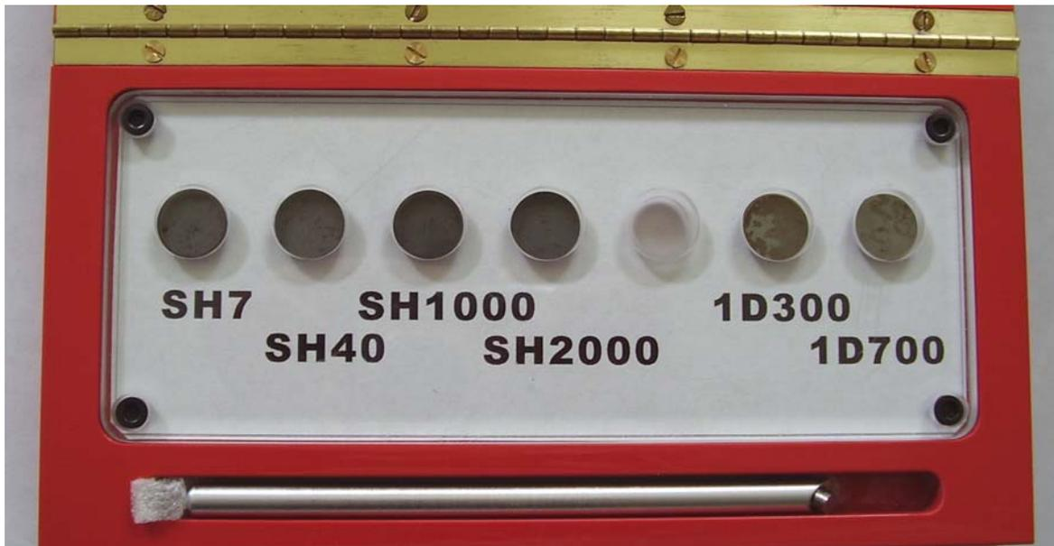
Fig. 6: A photograph of the box with the standards and the tool for handling (magnetic stick). In the normal position the back of the sample holder (steel disk  $\varnothing \sim 12\text{mm}$ ) can be seen, while the standard's reference side faces to the bottom.
