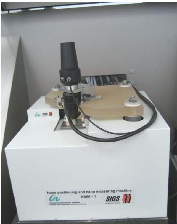
Fig. A3: Large range metrological atomic force microscope (LRM-AFM) consisting of a Nano Measuring Machine (NMM) and a commercial AFM head.
