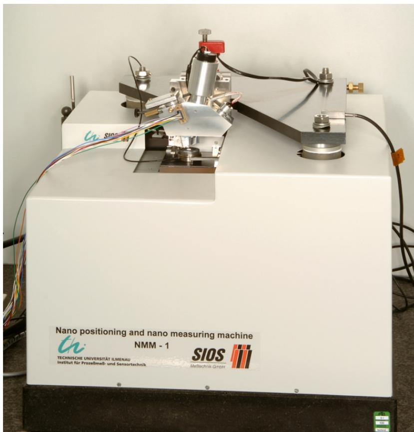
Fig. A4: Photo of the metrological large range SFM consisting of a Nano-Measuring-Maschine (NMM) and a home-built SFM head, described in [2]
