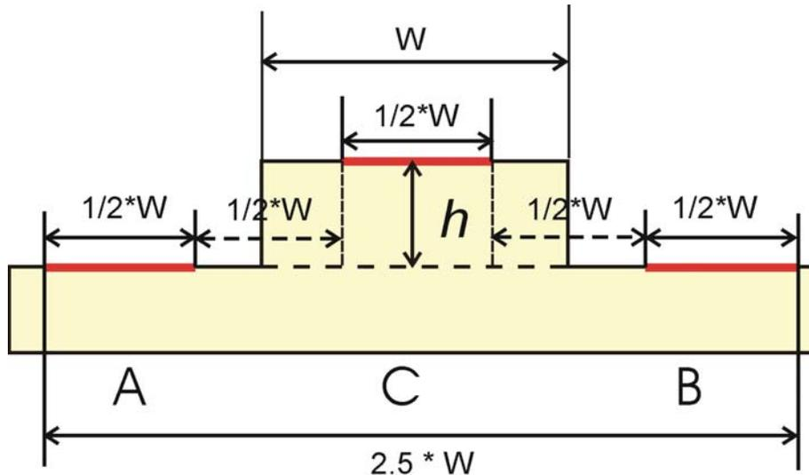
Fig. 8: Definition of step height  $h$  used in the comparison
