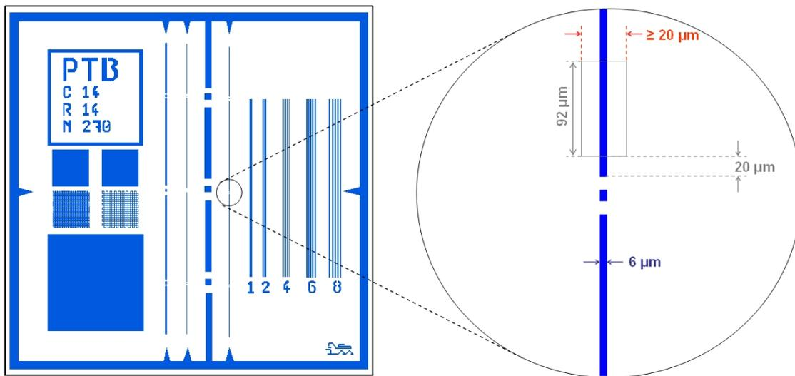
Fig. 1: Layout of the step height standards of 7 nm, 40 nm, 1000 nm, and 2000 nm step height. The substrate is silicon, the lines are silicon oxide, and the whole sample is covered by a chromium layer (not shown). There are four lines at the centre with widths of 20  $\mu\text{m}$ , 3  $\mu\text{m}$ , 100  $\mu\text{m}$  and 6  $\mu\text{m}$ . The line used for the comparison has a width of 6  $\mu\text{m}$  and is located on the right side.
