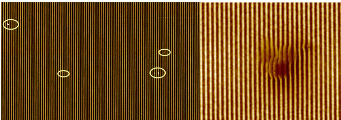
Fig. 5: Left: Minor particles on the 1D700 (SFM image); Right: Defect in the grating structure (here: SFM image of the 1D300)
