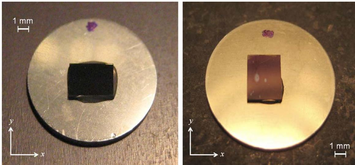
Fig. 3: Overview photographs of the lateral standards. Left: 1D300, right: 1D700.
