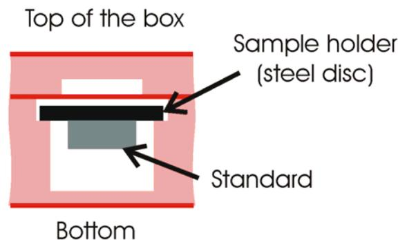
Fig. 7: Sketch showing the position of a standard in the box. Note: the structures are on the side facing downwards.
