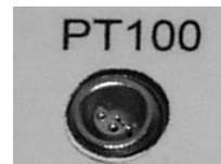
Figure 21 LEMO socket for measurement of the internal temperature: R_{PT100} .
