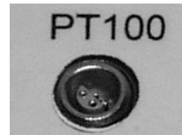
Figure 5. LEMO socket for measurement of the internal temperature: R_{PT100} .
