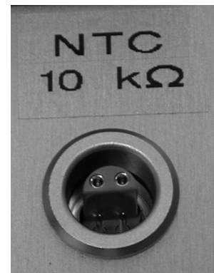
Figure 12 4-terminal LEMO socket for measurement of the internal temperature R_{NTC} of the thermostat.
