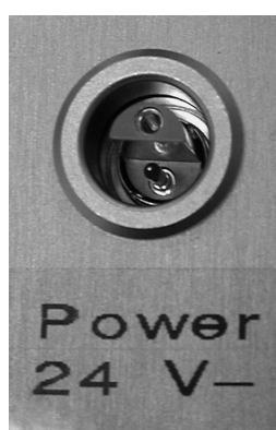
Figure 11. 2-terminal LEMO socket for the 24 V DC power supply of the thermostat.
