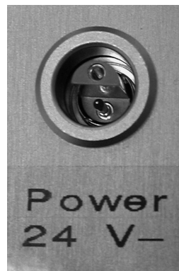
Figure 11 2-terminal LEMO socket for the 24 V DC power supply of the thermostat.
