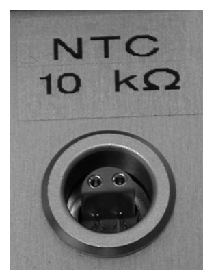
Figure 12. 4-terminal LEMO socket for measurement of the internal temperature R_{NTC} of the thermostat.
