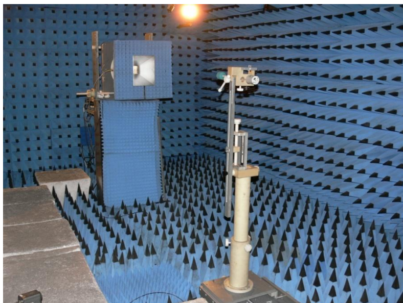
Figure 2 1.4 GHz – 18 GHz power flux density standard in the fully anechoic chamber
