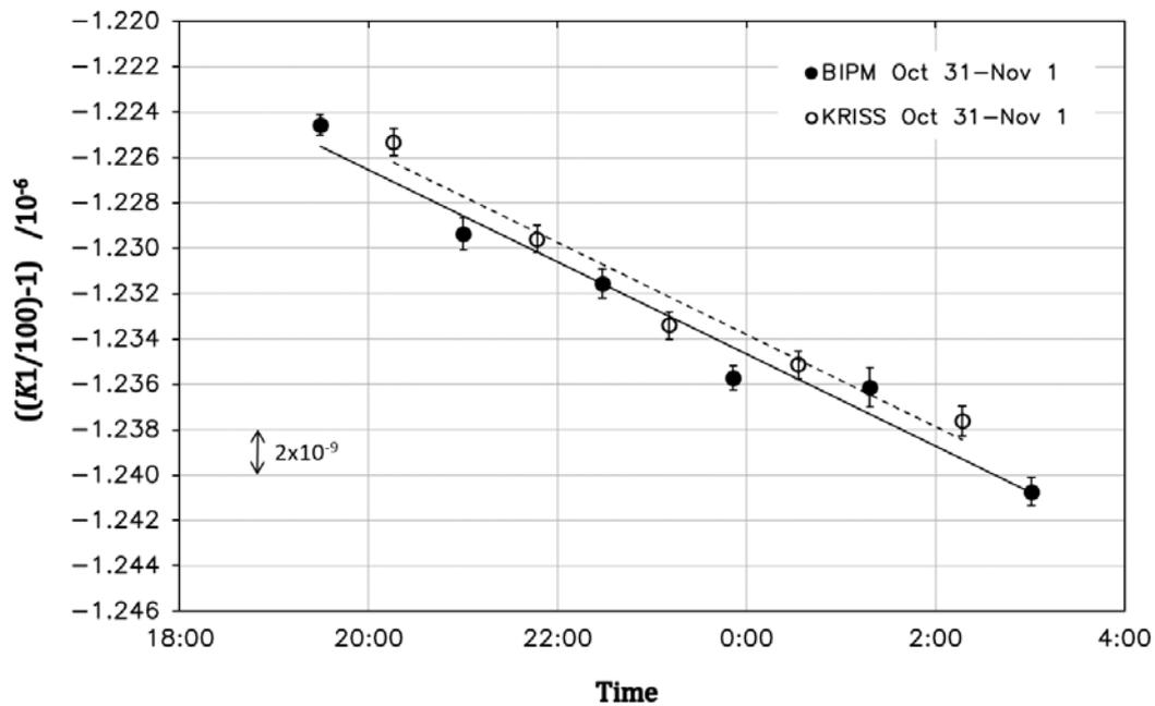
Figure 5: KRISS (open circles) and BIPM (black dots) corrected measurements of the ratio  $K1$  on October 31 – November 1, 2019. The error bars correspond to the dispersion observed during each measurement. Solid and dotted lines correspond to the linear fits of the BIPM and KRISS sets of measurements, respectively.
