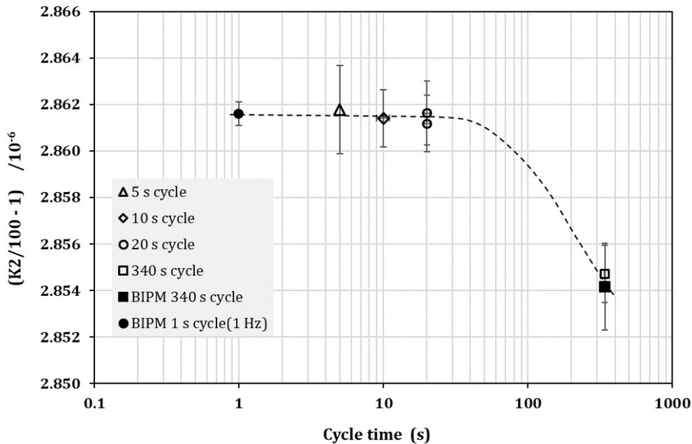
Figure 7: Preliminary measurements of the ratio  $K2$  performed by KRISS when the current reversal cycle time is varied from 5 s to 340 s. The dotted line is just a guide for the eye.
