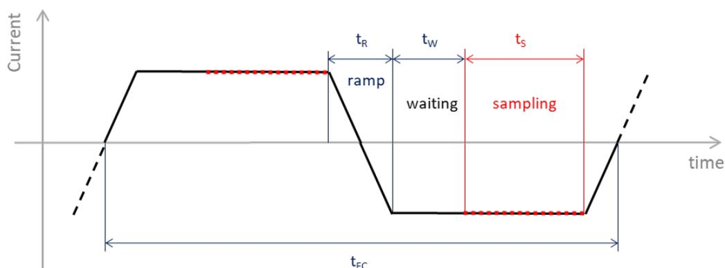
Figure 3: Current reversal timing of the KRISS measurement.  $t_R$ ,  $t_W$ ,  $t_S$ , and  $t_{FC}$  are the ramp time, waiting time, sampling time, and full cycle time, respectively
