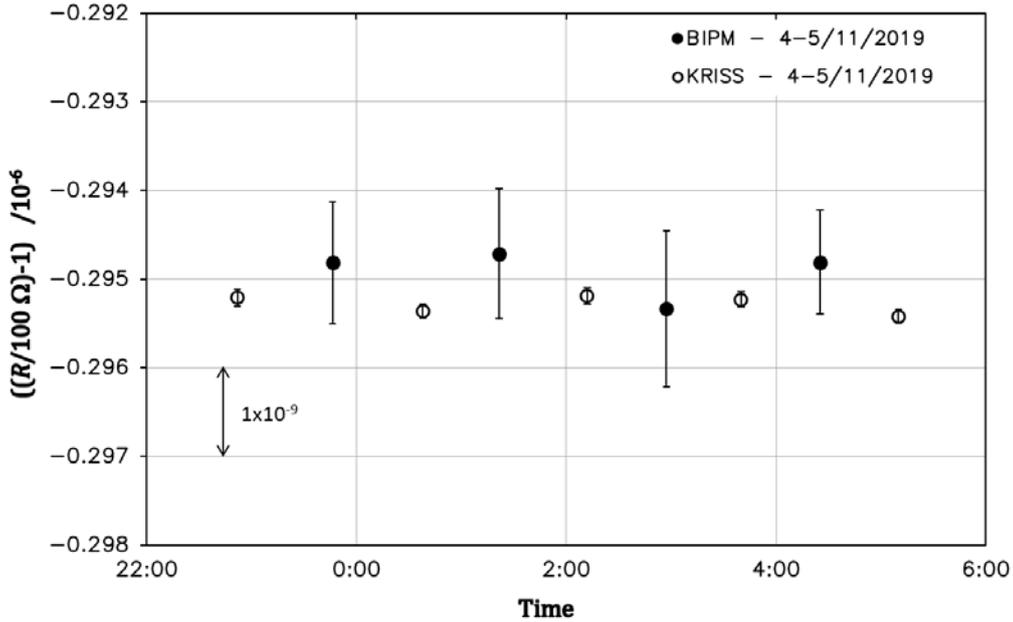
Figure 4: KRISS (open circles) and BIPM (black dots) corrected measurements of the 100 Ω resistance  $R_{100\Omega}$  in terms of  $R_H(2)$  on November 4-5, 2019. The error bars correspond to the dispersion observed for each measurement.
