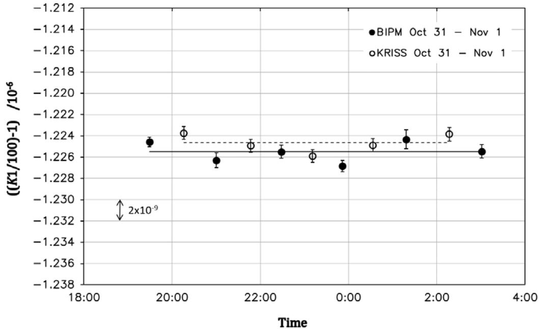
Figure 6: Same as Figure 5 but for BIPM and KRISS measurements corrected from the linear drift. Solid and dotted lines correspond to the linear fits of the BIPM and KRISS sets of measurements, respectively.
