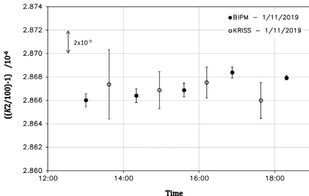
Figure 8: Measurement results for  $K2$  ratio on November 1, 2019: BIPM at 1 Hz (black dots) and KRISS for a 5 s cycle time (open circles). Error bars correspond to the dispersion observed for each measurement.
