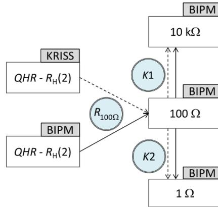
Figure 1: Schematic of the on-site comparison carried out at the KRISS in October-November 2019. Rectangles represent the resistances to be compared and circles correspond to the resistance  $R_{100\Omega}$  or the ratios  $K1$  and  $K2$  to be measured. Solid and dashed arrows stand for the measurements with the 1 Hz bridge of the BIPM or with the CCC bridge of the KRISS, respectively.
