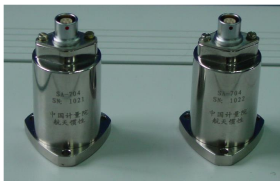
Figure 1: Two transfer standard accelerometers
