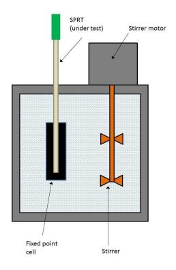
Figure 5. Typical stirred liquid bath.
