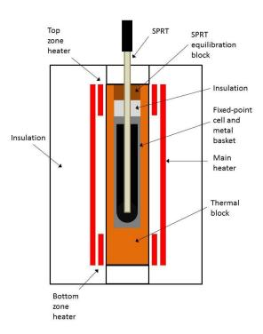
**Figure 6.** Medium temperature three-zone furnace for resistance thermometry metal freezing points.
