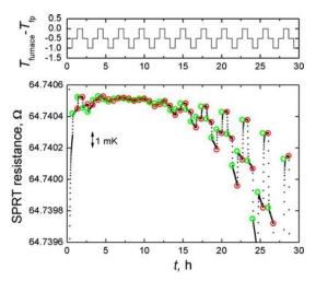
**Figure 10.** SPRT resistance as a function of time during Zn freeze, while the furnace temperature is oscillating by ±0.5 K, indicating a penetration ratio of ~0.01. *Illustration reproduced with the permission of Springer: International Journal of Thermophysics,* "A New Method for the Quantification and Correction of Thermal Effects on the Realization of Fixed Points", vol. **29**, 2008, pp. 126-138, authors: M. Fahr and S. Rudtsch.
