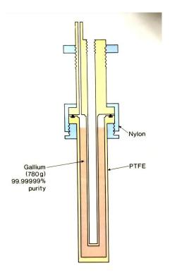
Figure 2. Gallium melting and triple-point cell.
