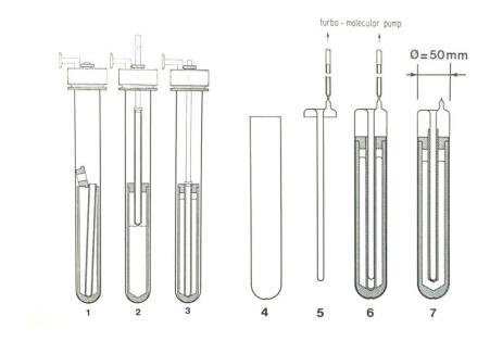
**Figure 4.** Preparation and filling of a sealed cell suitable for the freezing points of In, Sn, Zn, Al, and Ag [Nubbemeyer (1990)]: (1) Parts ready for baking in vacuum. (2) Join the graphite parts and the metal block (or shot) of the fixed-point cell. (3) Melt the metal block and lower the graphite well completely. (4) and (5) Quartz parts ready for degreasing. (6) Assemble crucible and quartz parts, seal the quartz, evacuate and fill with argon. (7) Seal off.
