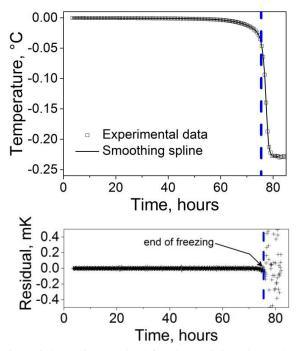
**Figure 12.** Illustration of the spline method for determining the end-point of a freeze. The appearance of 'noise' (i.e. residuals in the spline fits) suggests that the endpoint is at about 76.4 h. [Pearce *et al.* (2013)]<sup>4</sup>. Note that the end-point of freezing occurs at a temperature way below the plateau (this is also the case for the heater power determination of the end-point in Figure 11).
