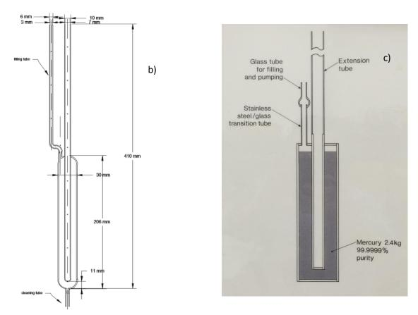
**Figure 1**. Distillation apparatus for mercury cells (a), and design (b) [del Campo *et al.* (2008)]. c) Stainless-steel mercury cell. *Illustration reproduced with the permission of Springer: International Journal of Thermophysics, "Assembly and Study of Different Mercury Cells with Known Impurity Content and Isotopic Composition", vol. 29, 2008, pp. 93-103, authors: D. del Campo, V. Chimenti, J. Reyes, J.A. Rodriguez Castillon, M. Moldovan and J.I. Garcia Alonso.*
