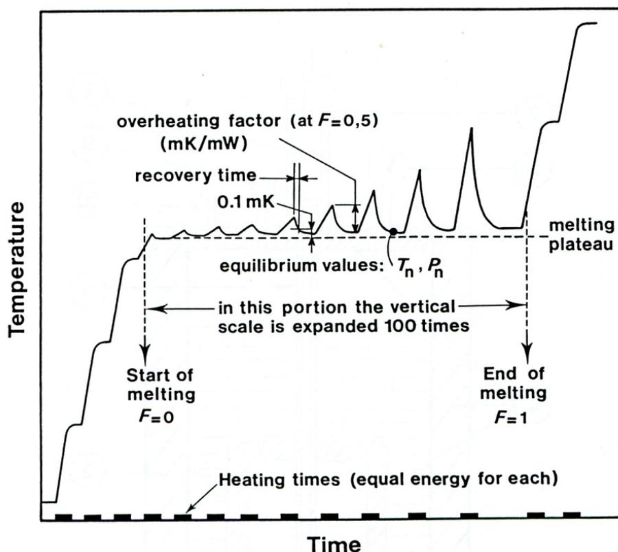
**Figure 8.** A schematic representation of melting a fixed-point sample by intermittent heating (after Pavese (1984)). Heating is supplied in equal-energy steps.  $F$  is the melted fraction. The melting lasts at least several hours.
