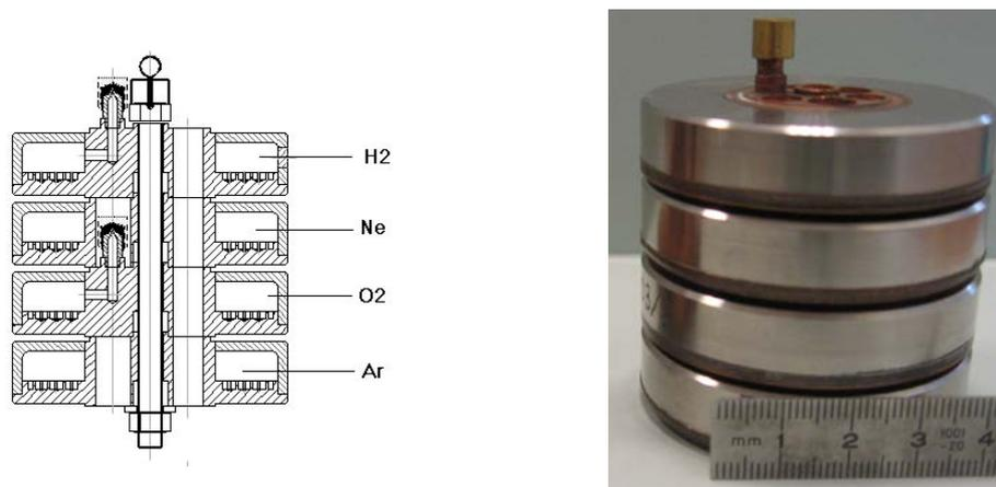
**Figure 3.** Sealed-cell model developed at LNE-Cnam after 1990 within the framework of an international collaboration, reproduced from [Hermier *et al.* 2003, Pavese *et al.* 2003a] with the permission of AIP Publishing: On the left (not to scale): Schematic diagram of an assembly composed of four cells for the realization of the triple points of hydrogen, neon, oxygen, and argon, pressed together with the central screw. On the right: Photograph of an assembly with four cells.
