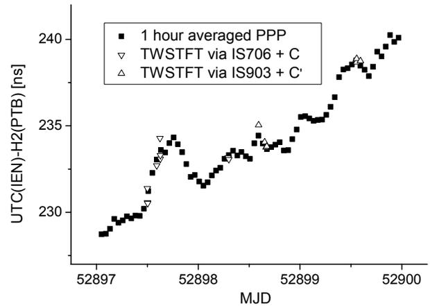
Figure 6. H2(PTB)-UTC(IEN) as evaluated with TWSTFT and PPP.
