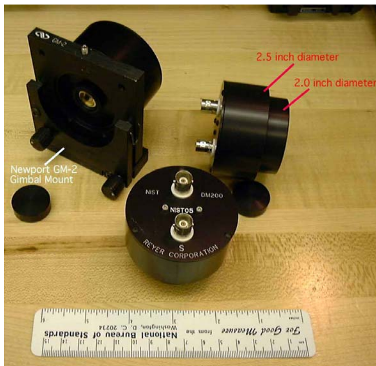
Figure 2.1. InGaAs photodiode mounted in package used for the key comparison.
