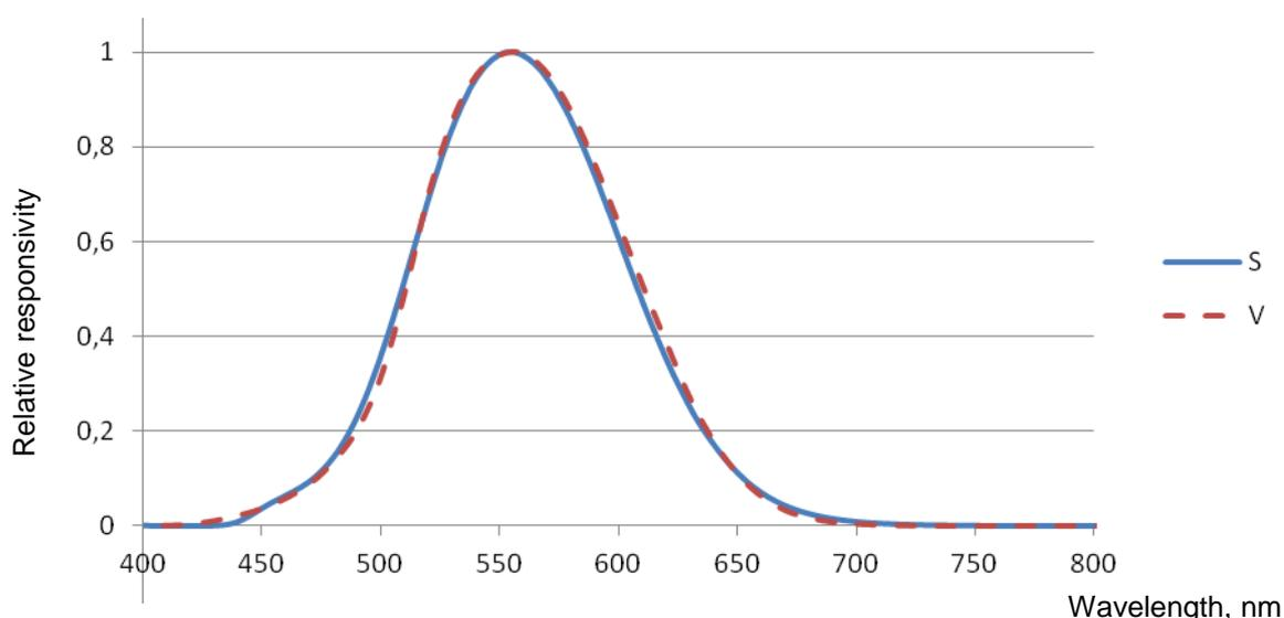
Figure 4. Relative spectral responsivity of the primary photometer -  $S(\lambda)$  and the luminosity curve -  $V(\lambda)$ .
