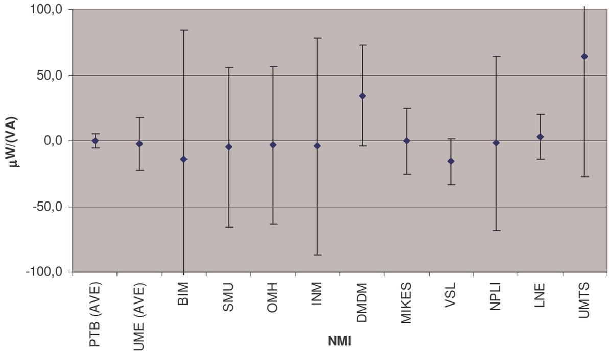
Figure 9. Deviation from Reference Value 120 V, 5 A, PF=0.0 Lead (k=2)
