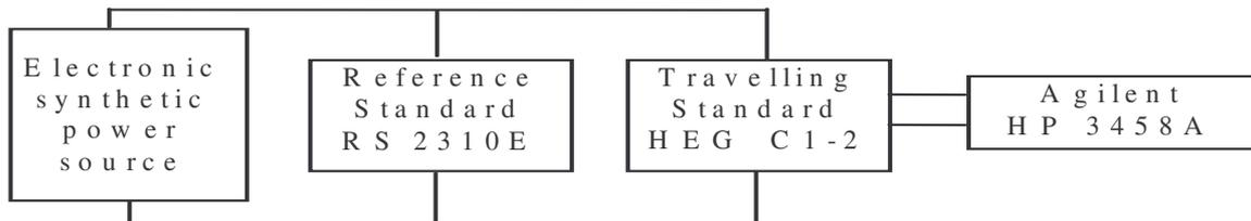
The DC output voltage of the travelling standard is measured using the digital voltmeter Agilent-HP 3458A, which has been calibrated with dc voltage standard immediately before the test.
