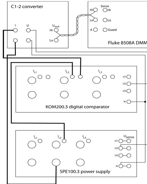
Block diagram of the calibration set-up.
