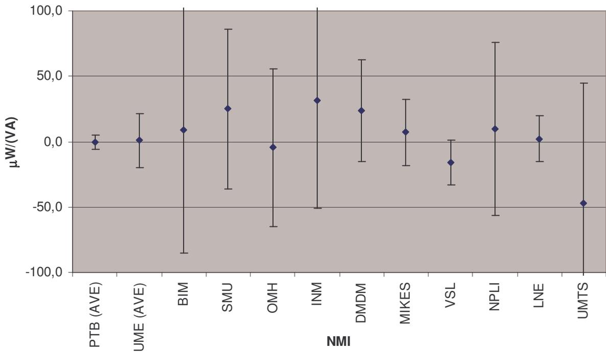
Figure 8. Deviation from Reference Value 120 V, 5 A, PF=0.5 Lag (k=2)
