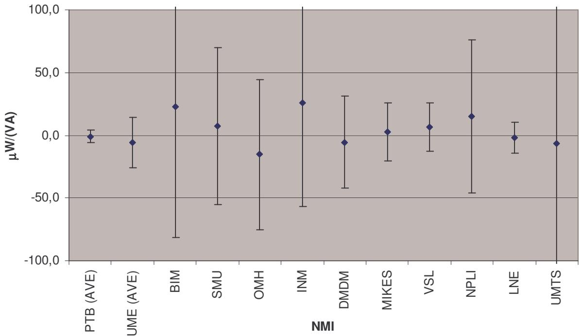
Figure 10. Deviation from Reference Value 120 V, 5 A, PF=0.0 Lag (k=2)
