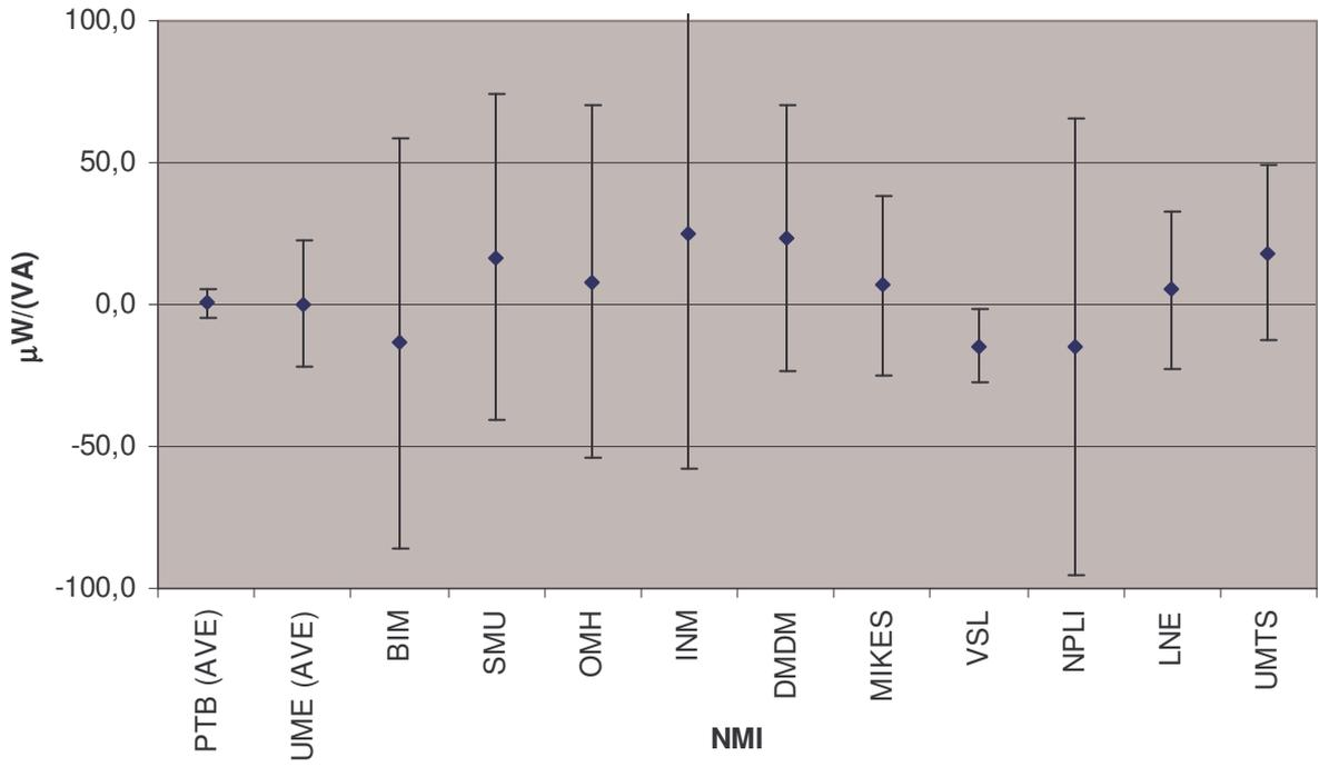
Figure 7. Deviation from Reference Value 120 V, 5 A, PF=0.5 Lead (k=2)
