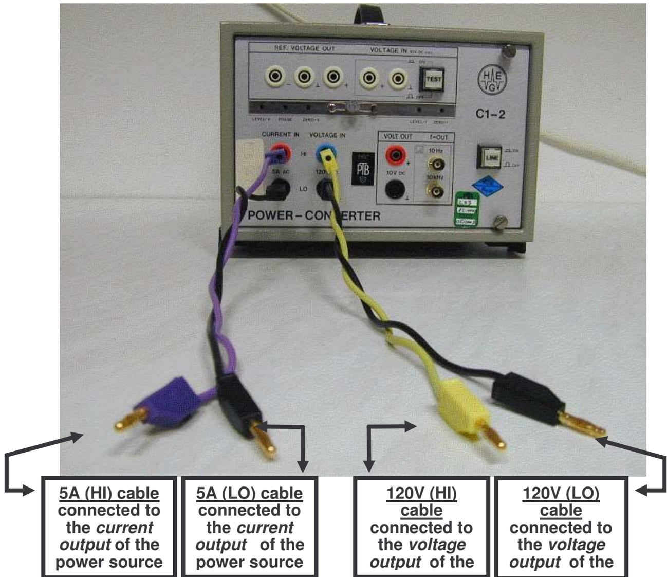
**Figure 2.** Current and voltage input connections of the travelling standard.
