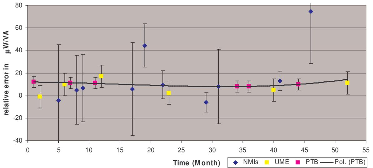
Figure 4. Reported Results, 120 V, 5 A, PF=0.0 Lead (cap) (k=1)
