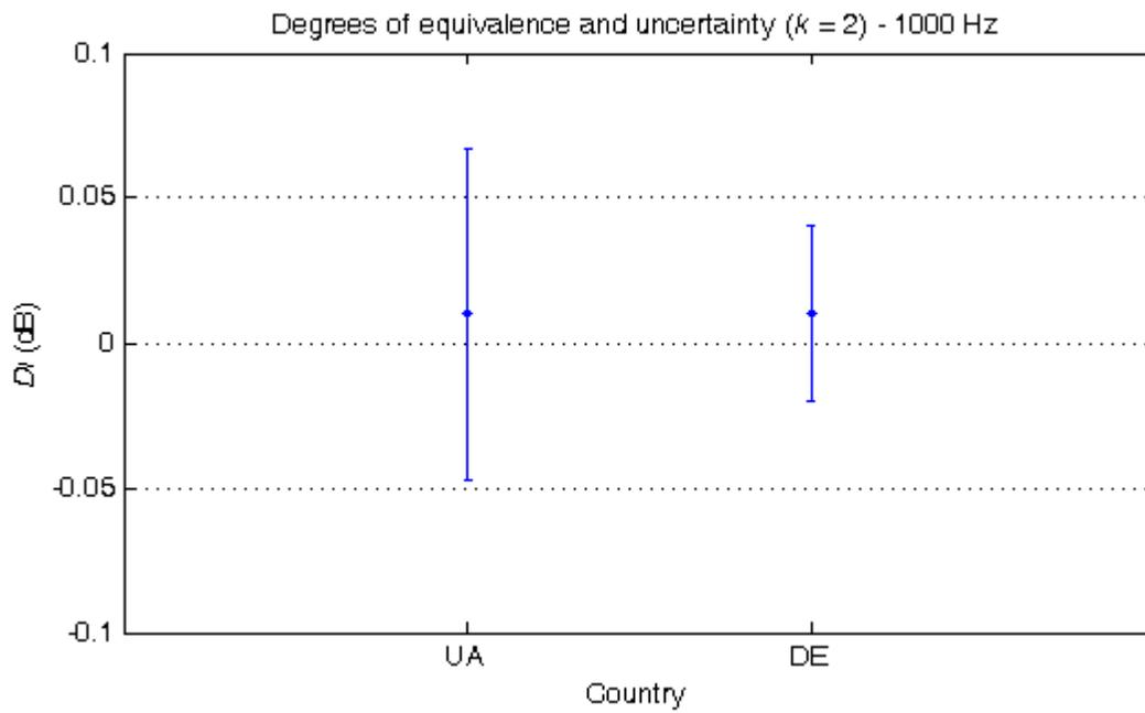
**Fig. 5** Degrees of equivalence with the KCRV at 1000 Hz
