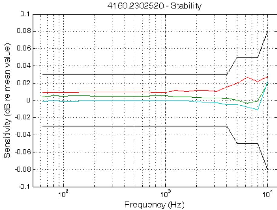
**Fig. 1** Stability of the travelling standard microphone 4160.2302520 measurements over frequency, compared to PTB uncertainty ( $k = 2$ ).
