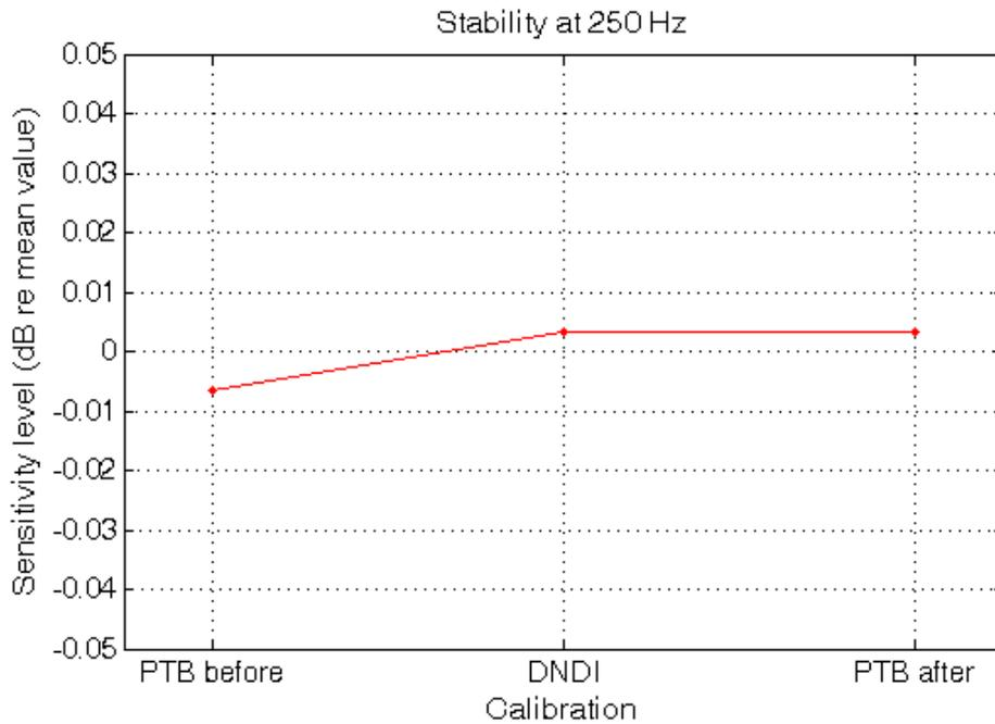
**Fig. 2** Typical variation with time at  $f = 250$  Hz for the travelling standard
