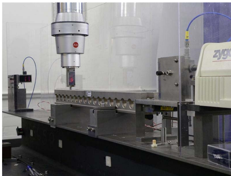
Fig 1. Measurement of a step gauge using the Step Gauge Rig mounted on the Leitz CMM
