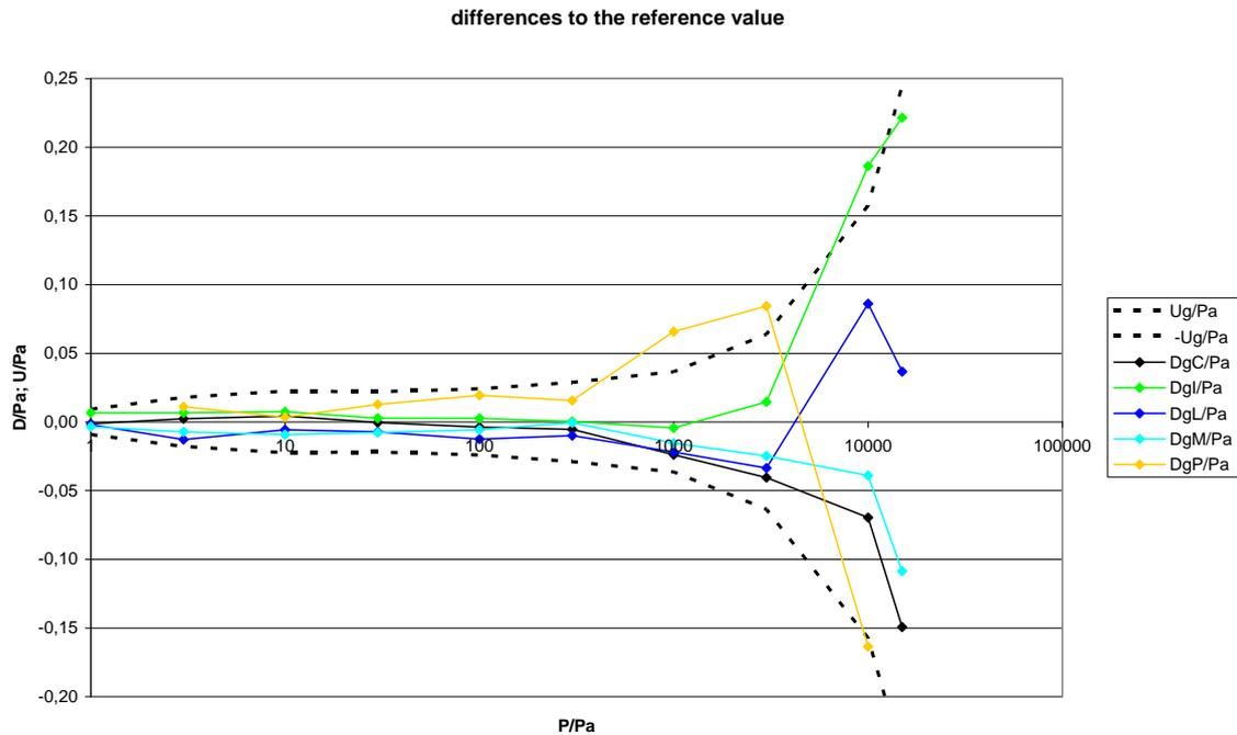
Fig. 10.1: Results to the reference value in gauge mode.
