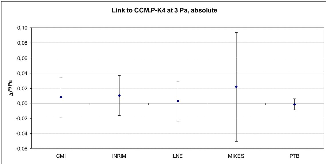
*Fig. 11.1: The differences to the CCM.P-K4 reference value at 3 Pa.*
