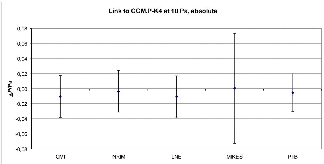
*Fig. 11.2: The differences to the CCM.P-K4 reference value at 10 Pa.*
