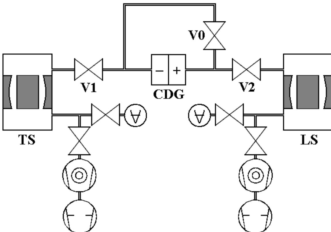
Fig. 8.2: Arrangement of the TS in the absolute mode.
