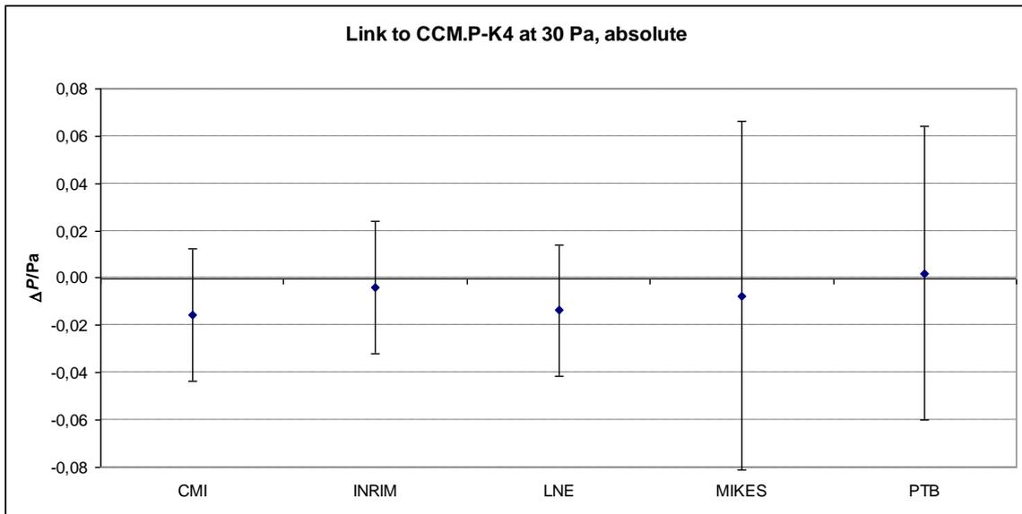
Fig. 11.3: The differences to the CCM.P-K4 reference value at 30 Pa.
