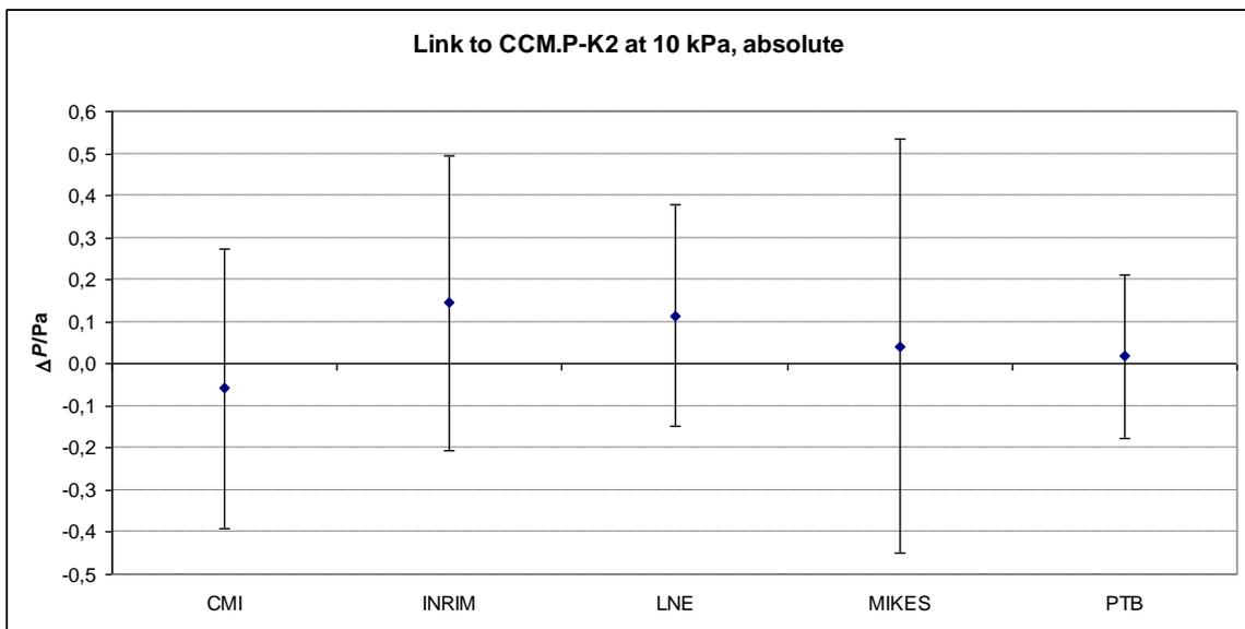
Fig. 11.4: The differences to the CCM.P-K2 reference value at 10 kPa.
