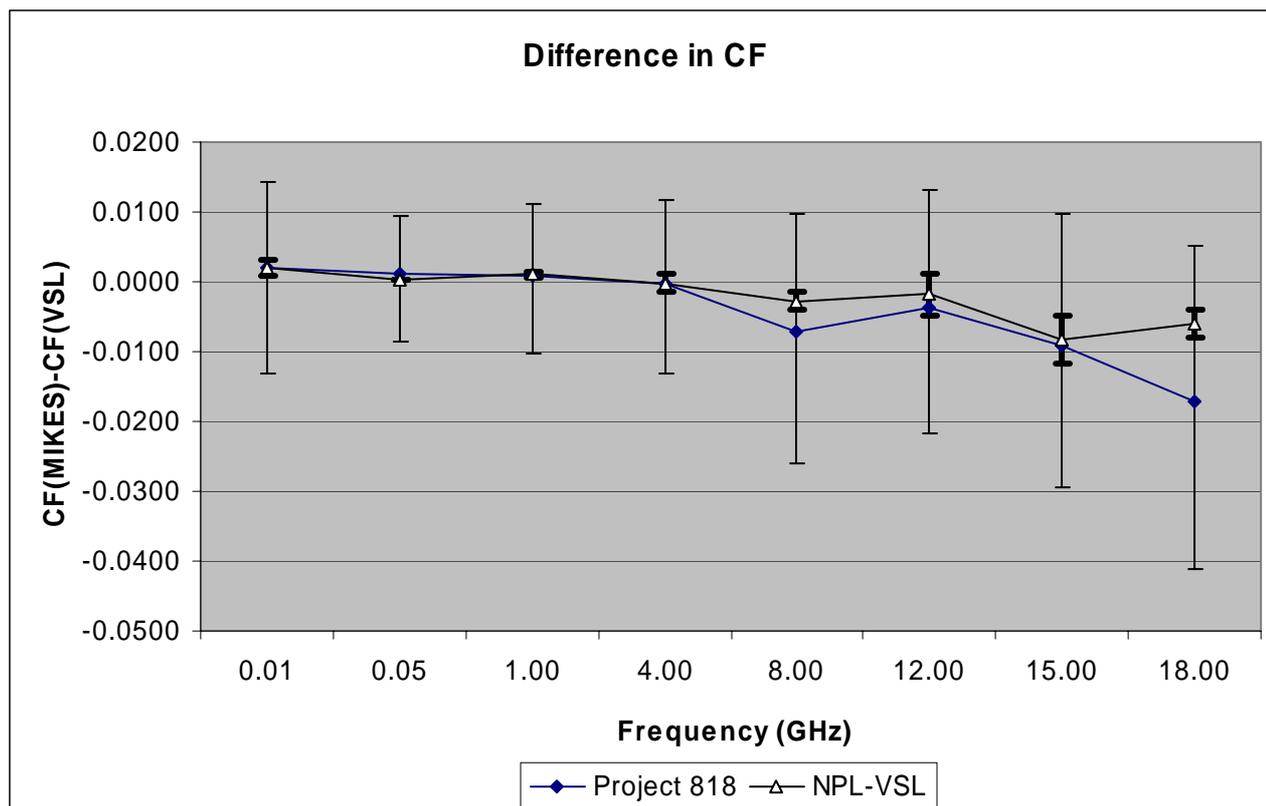
Figure 4: The data of project 818 refer to the measured difference in Calibration Factor between MIKES and NMi-VSL (using the data from Table 2). The data marked as “NPL-VSL” refer to similar results in project 633 between NPL and NMi-VSL (using the information from Table 3).
