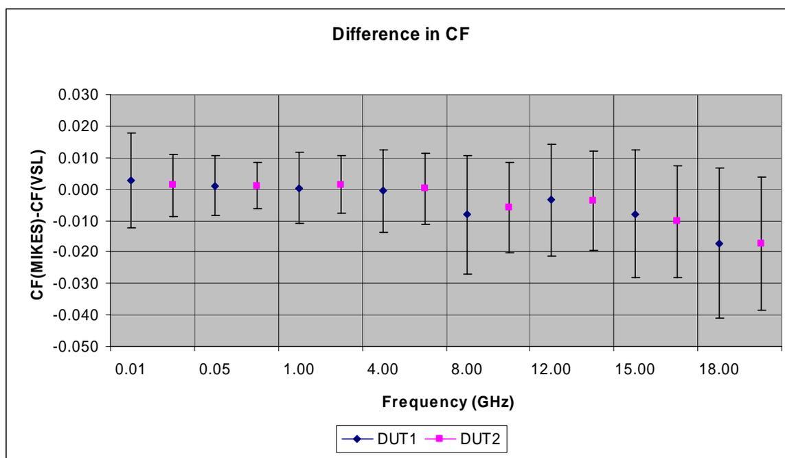
Figure 3: The difference in measured calibration factor as function of frequency. The calibration factor determined by the pilot is taken as reference. The error bars are based on the RSS value of the individual uncertainty budgets, using  $k=2$ .
