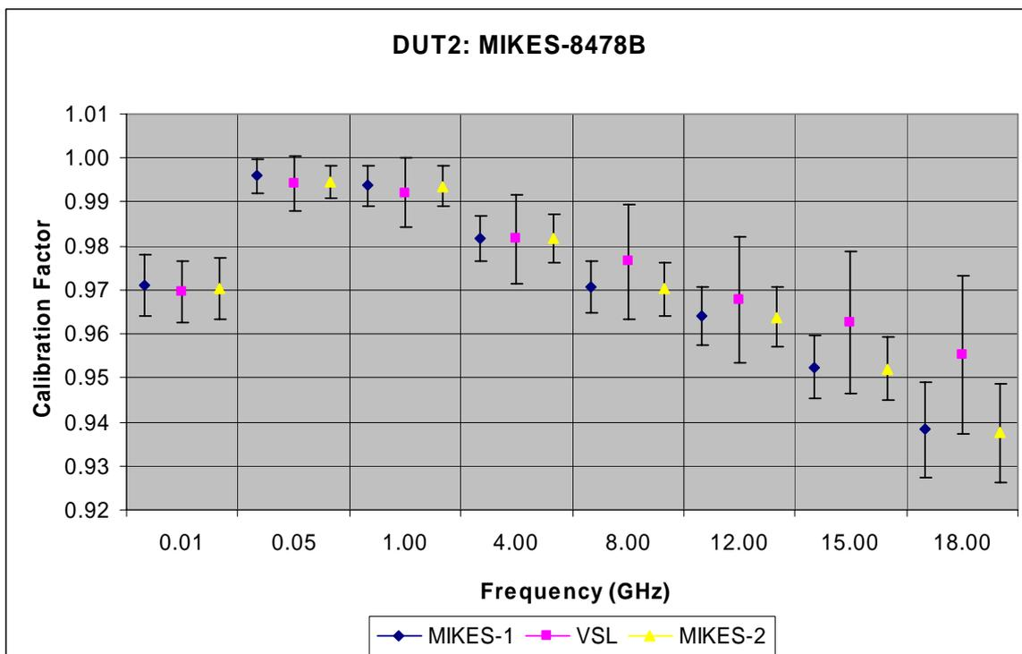
Figure 1: The calibration factor as function of frequency as determined by the two participants. Each laboratory has measured its own thermistor mount at the beginning and at the end of the comparison. The uncertainty bars refer to the expanded standard deviation ( $k=2$ ) in the results of the participants.
