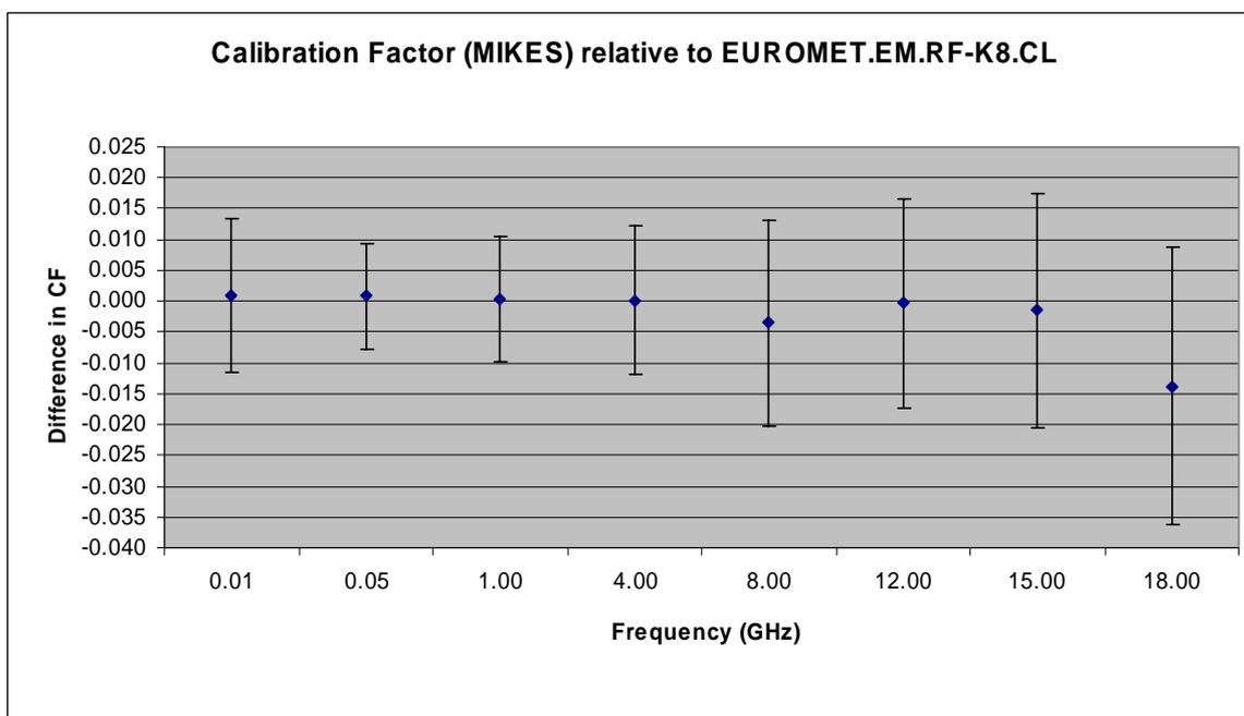
Figure 5: The average difference between the results from MIKES and the reference value obtained in the EUROMET.EM.RF-K8.CL
