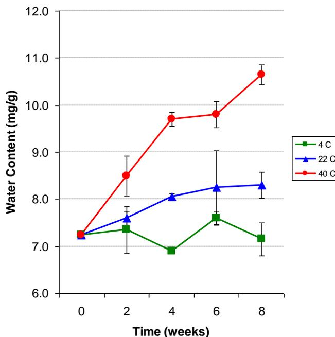
**Figure 2: Effect of storage temperature on water content for CCQM-K55.a**
