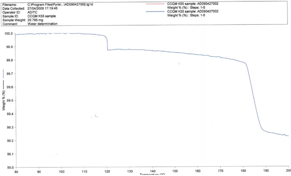
TGA data for CCQM-K55.a in range 80 °- 200 °C showing an initial mass loss (ca 1.5 mg/g, 0.15 % relative) at 120 °C and subsequent mass loss (ca 6 mg/g) above 170 °C
