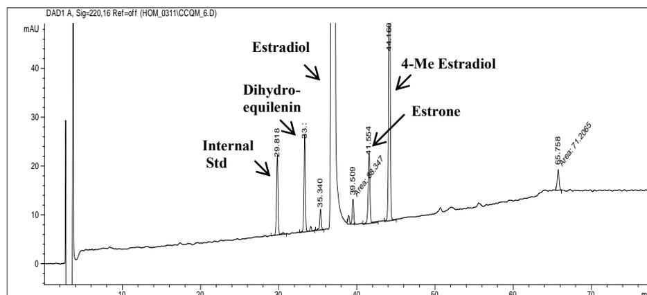
**Figure 3b: Artefact formation suppressed in LC-UV chromatogram of CCQM-K55.a at 220 nm when eluting with acidified (0.05% TFA) solvent**
