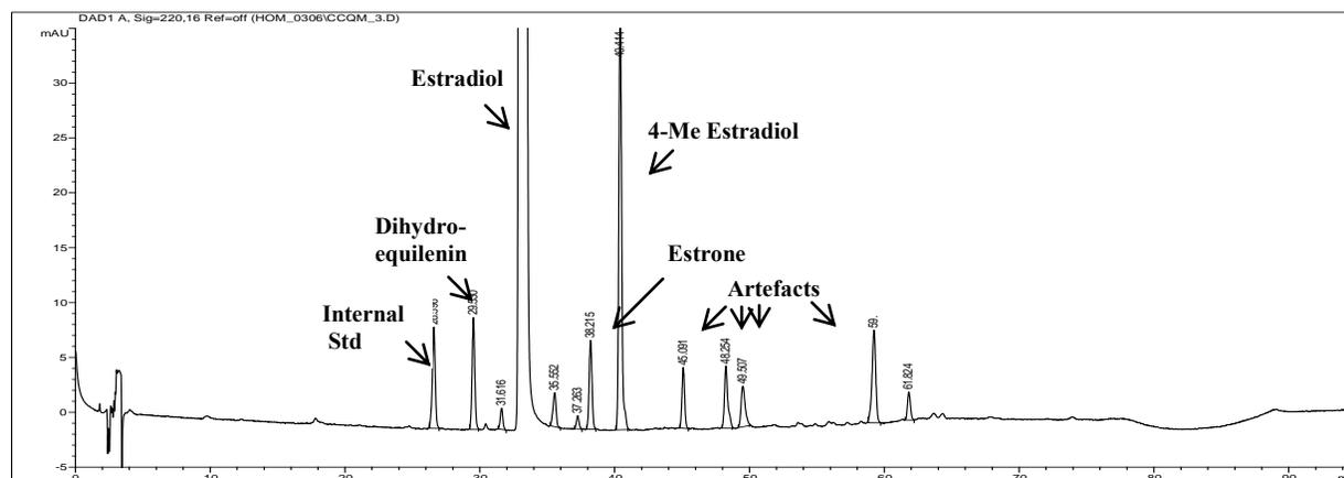
**Figure 3a: Artefact formation visible in LC-UV chromatogram of CCQM-K55.a at 220 nm when eluting with neutral aqueous solvent**
