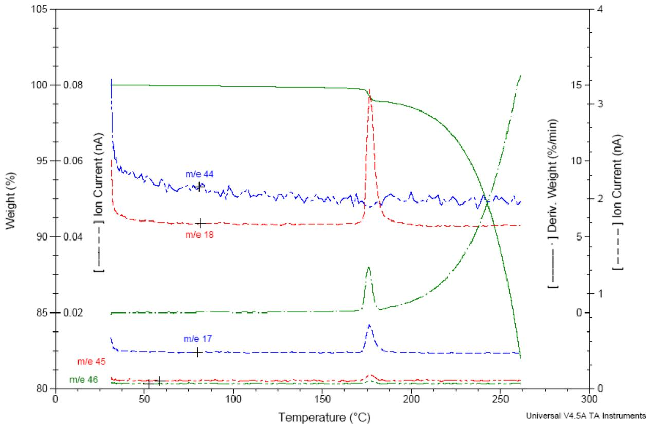
TGA-MS of CCQM-K55.a in range 30 °C – 250 °C showing mass loss (solid green line), mass change derivative (alternating green lines) at 170 °C and ion current (dashed lines) for selected  $m/z$  from liberated volatile material
